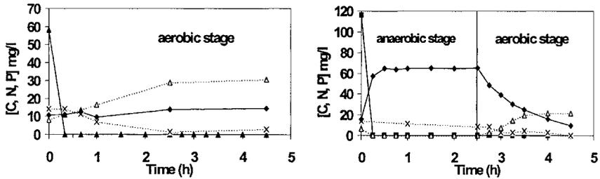
**Figure 2** Soluble C, N and P concentrations during one cycle of the non P-accumulating (left) and the P-accumulating (right) parent reactors.  $\blacktriangle$ : AGV; X:  $N-NH_4$ ;  $\triangle$ :  $N-NO_3$ ;  $\blacklozenge$ :  $P-PO_4$
