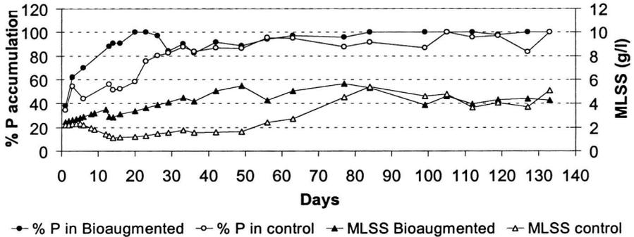
**Figure 3** Evolution of the MLSS (mixed liquor suspended solids) and P accumulation in the bioaugmented and control reactors with time. T0 corresponds to the day of bioaugmentation
