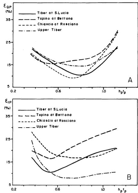
Fig. 3. Nash method. A) Mean value of the peak flow error as a function of the product of the IUH peak flow and its time to peak. B) Mean value of the time to peak error as a function of the product of IUH peak flow and its time to peak.
