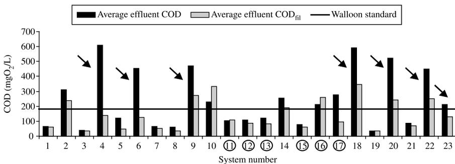
**Figure 5** | Average COD (dark bars) and COD<sub>fil</sub> (light bars) of the effluent of the 23 systems, accompanied by the Walloon standard. The circled system numbers 11, 12, 13, 15, 16 and 17 are situated in the Walloon region, the others are situated in Flanders. The arrows point out the great difference between the COD and COD<sub>fil</sub>, possibly induced by a wash out situation.
