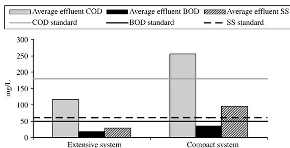
**Figure 6** | Comparison of the average effluent BOD, COD and SS values of compact and extensive systems. The lines represent the different standards.
