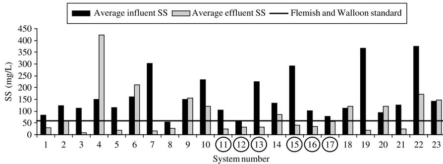
**Figure 4** | Average SS of influent (dark bars) and effluent (light bars) of the 23 systems, accompanied by the Flemish and Walloon standard. The circled system numbers 11, 12, 13, 15, 16 and 17 are situated in the Walloon region, the others are situated in Flanders.
