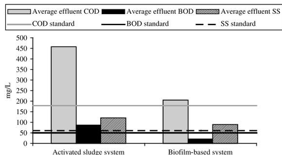
**Figure 7** | Comparison of the average effluent BOD, COD and SS values of suspended growth and attached-growth systems. The lines represent the different standards.
