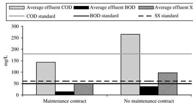
**Figure 8** | Comparison of the average effluent BOD, COD and SS values of systems with and without a maintenance contract. The lines represent the different standards.
