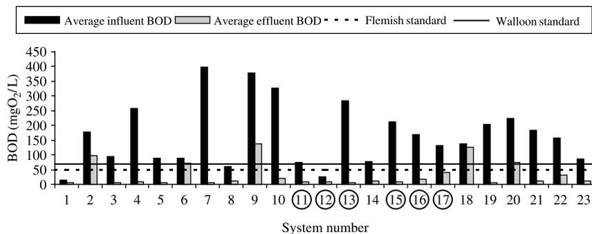
**Figure 2** | Average BOD of influent (dark bars) and effluent (light bars) of the 23 systems, accompanied by the Flemish and Walloon standard. The circled system numbers 11, 12, 13, 15, 16 and 17 are situated in the Walloon region, the others are situated in Flanders.
