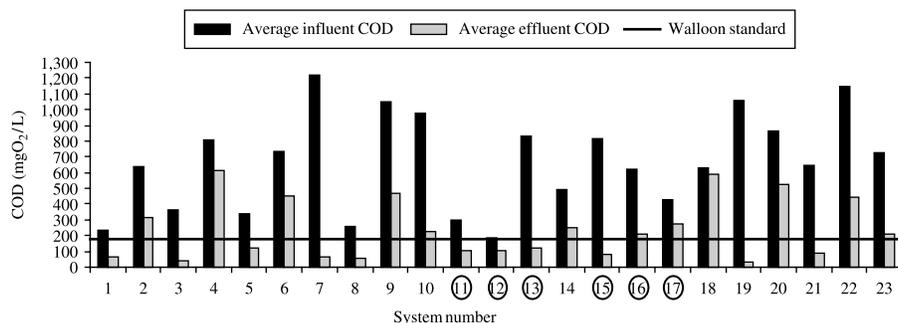
**Figure 3** | Average COD of influent (dark bars) and effluent (light bars) of the 23 systems, accompanied by the Walloon standard. The circled system numbers 11, 12, 13, 15, 16 and 17 are situated in the Walloon region, the others are situated in Flanders.
