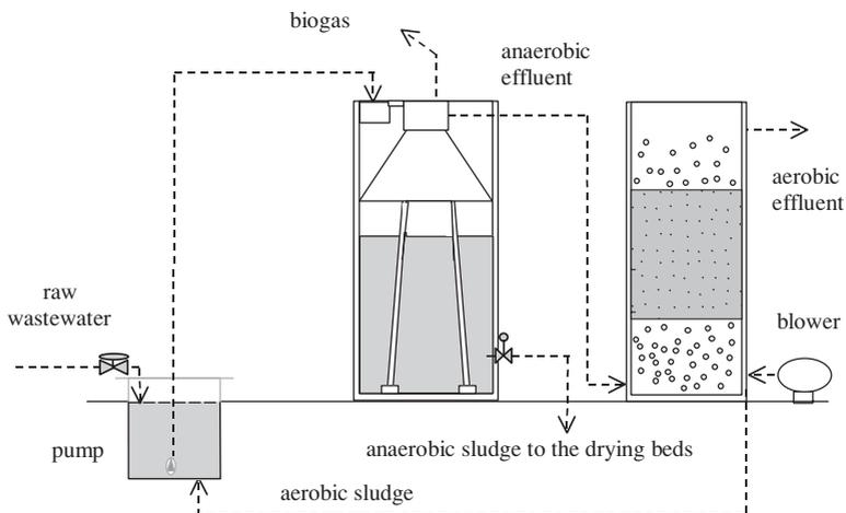
**Figure 1** Flow diagram of the UFES WWTP
