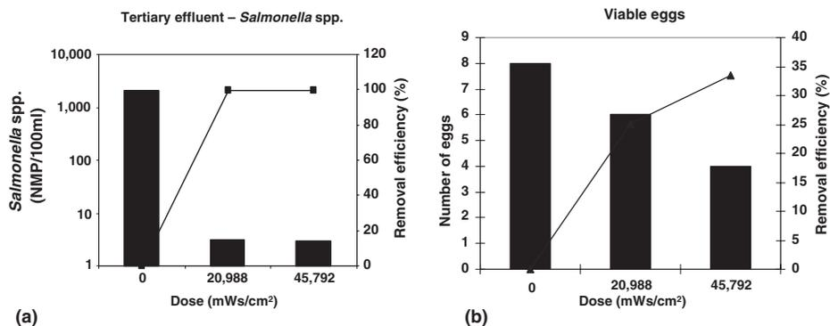
**Figure 4** Removal of *Salmonella* spp. (a) and helminth eggs (b) after increasing doses of UV irradiation at three points in the UV reactor
