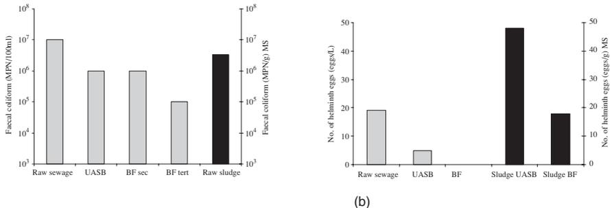
**Figure 2** Thermotolerant coliform density (a), and helminth egg counts (b), detected in the liquid phase and in the solid phase of the treatment at WWTP
