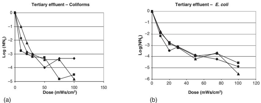
**Figure 3** Inactivation of coliforms (a) and *E. coli* (b) present in the tertiary effluent after increasing doses of UV irradiation
