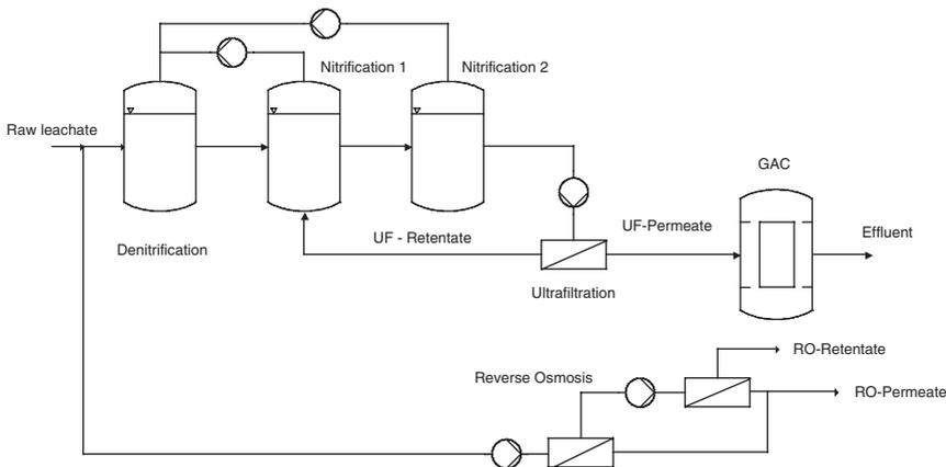
**Figure 3** Membrane bioreactor configuration at a landfill leachate treatment plant
