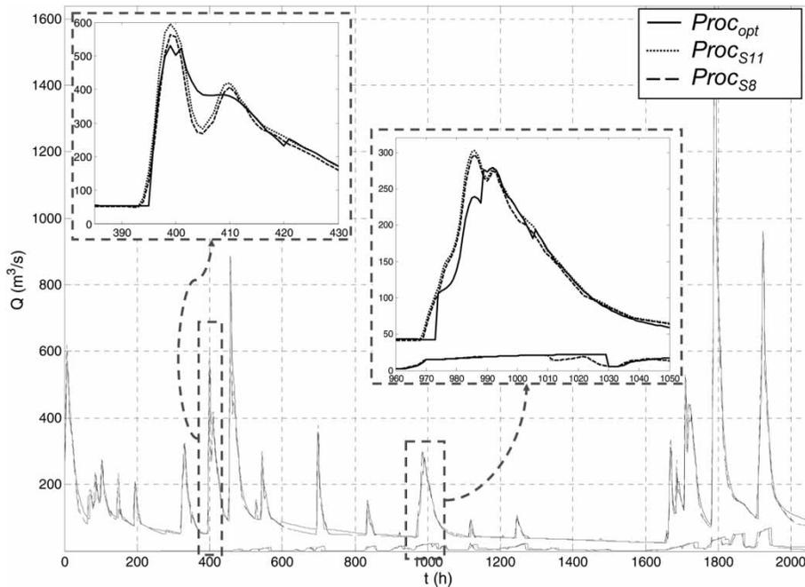
**Figure 7** | Comparison between the band obtained using the procedure for solving the direct problem, described in Simulation of the rainfall-runoff process using the grey ADM model ( $Proc_{opt}$ ), and those obtained with the expeditious procedure considering  $n_{par} = 11$  parameters and only the  $n_{par}^* = 8$  most significant parameters.
