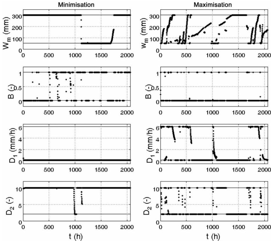
**Figure 6** | Crisp values (black dots) of the parameters  $W_m$ ,  $B$ ,  $D_1$  and  $D_2$  provided by the optimisation process for identification of the lower (left column) and upper (right column) extremes of the grey discharges for the period 5/12/1959–28/2/1960. The grey lines represent the lower and upper extremes of the grey numbers of the parameters within which the crisp numbers are sought (see Table 1).
