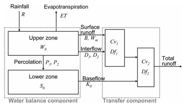
Figure 1 | Schematic representation of the ADM model.
