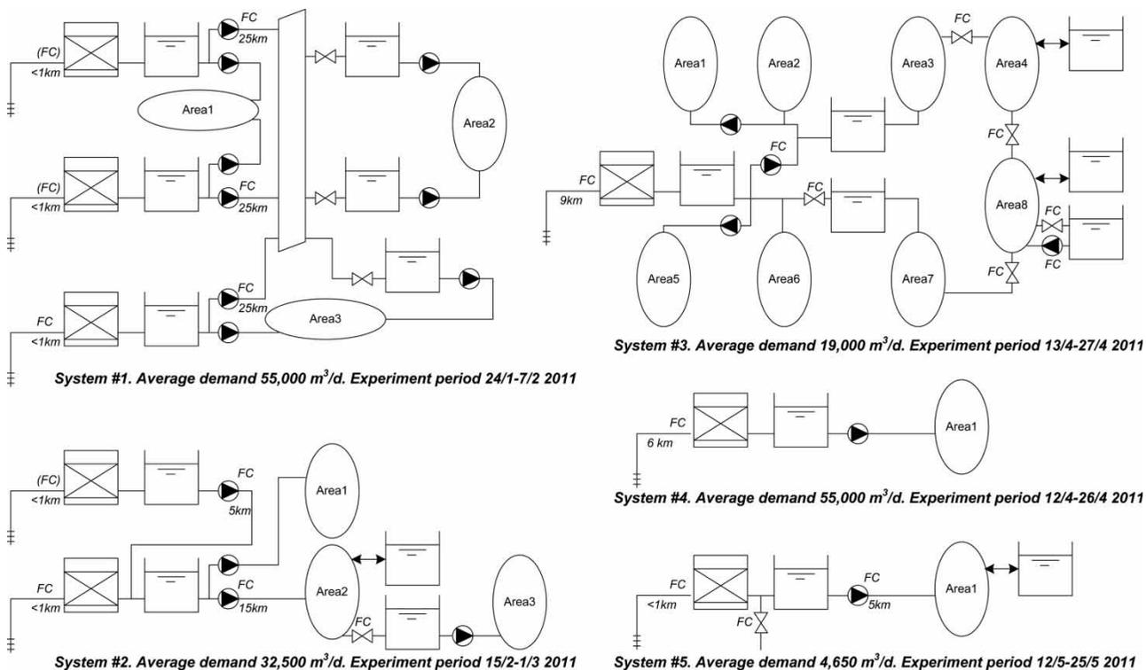
**Figure 3** | Configurations of the five examined water supply systems. The flow controlled elements are indicated by 'FC'. The elements indicated with '(FC)' are always level-based flow controlled (also when predictive flow control is active).
