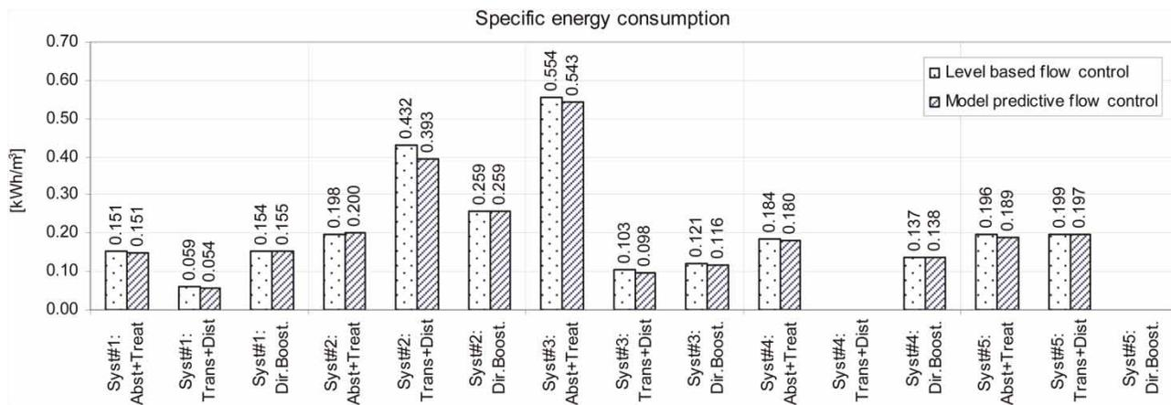
Figure 8 | Specific energy consumption per component of energy consumption for each system.
