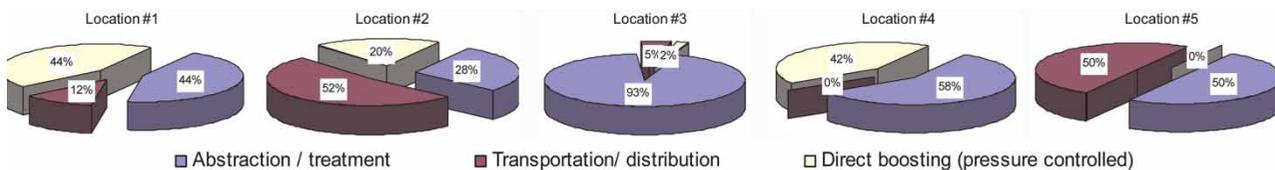
Figure 5 | Division of total energy consumption over the three components of energy consumption.
