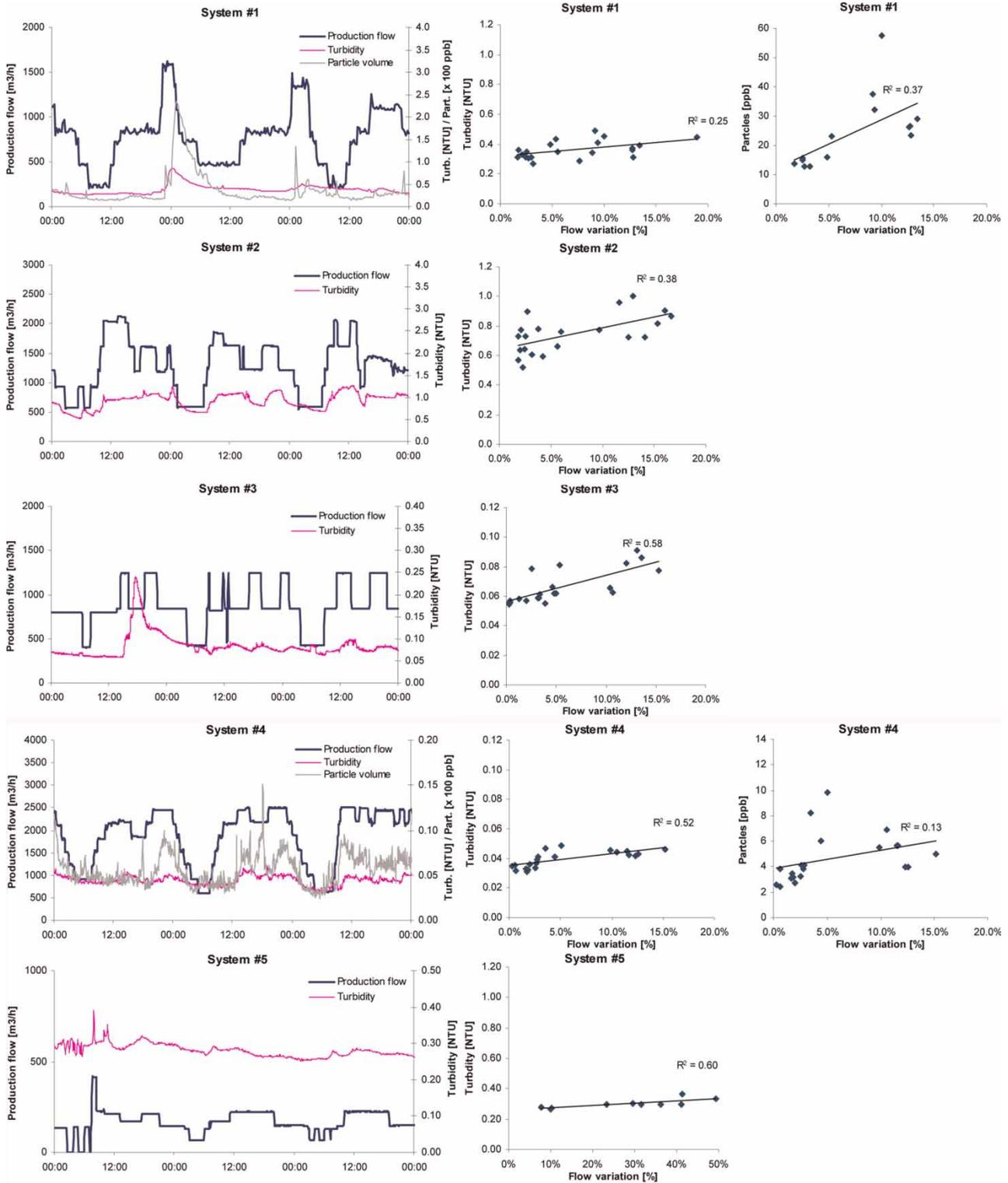
**Figure 7** | Relation between production flow variations and turbidity/particle volume in clear water, at systems controlled with predictive control. The graphs on the left show the turbidity and the flow variations in time. The graphs on the right show the relation between average daily values of flow variations and average daily values of turbidity (middle graphs) or particle volume (right graphs).
