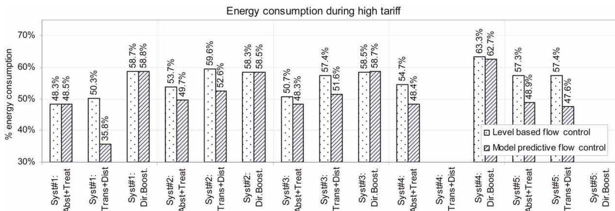
Figure 9 | Percentage of energy consumption during high tariff per component of energy consumption for each system.
