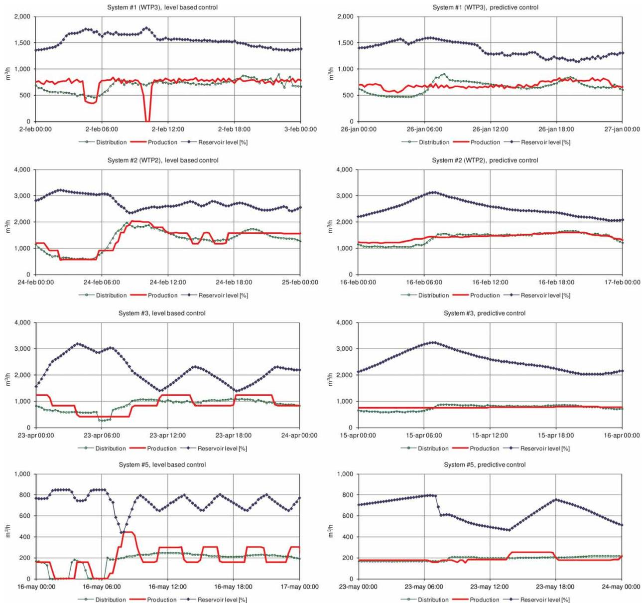
**Figure 6** | Trends of level-based control (left) and model predictive control (right).
