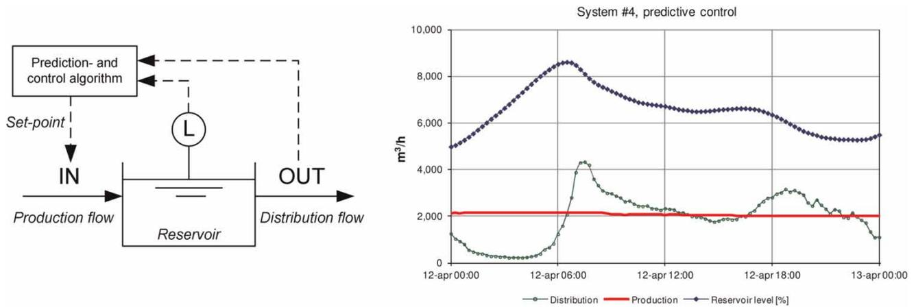
**Figure 2** | Principles of model predictive flow control and trends of production flow, distribution flow and level in the clear water reservoir on a day with model predictive flow control.
