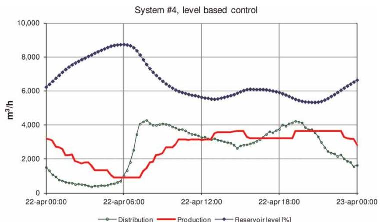
Figure 1 | Principles of level-based flow control and trends of production flow, distribution flow and level in the clear water reservoir on a day with level-based flow control.
