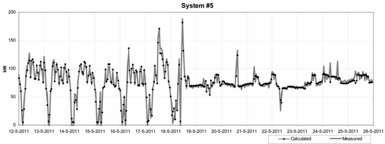
Figure 4 | Example of trend with calculated energy consumption and measured energy consumption.
