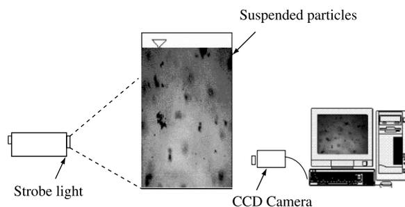
Figure 1 | Experimental setup for *in situ* particle characterization studies.
