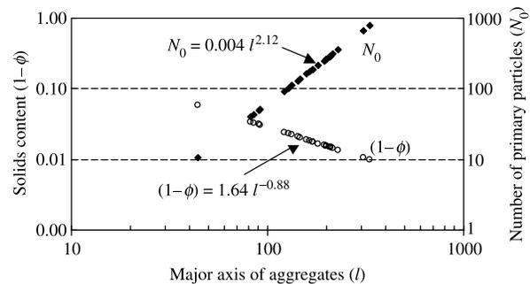
**Figure 6** | Solids content and number of primary particles contained in the aggregates. For solids content  $(1 - \phi)$ : median = 0.02, range = 0.01–0.06; for  $N_0$ : median = 408, range = 23–1700.
