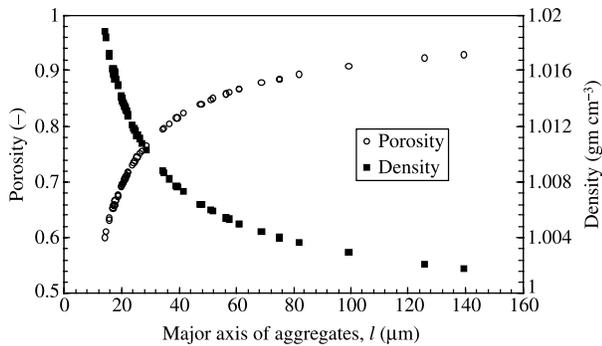
**Figure 5** | Aggregate properties as a function of size for measured data for density and porosity.
