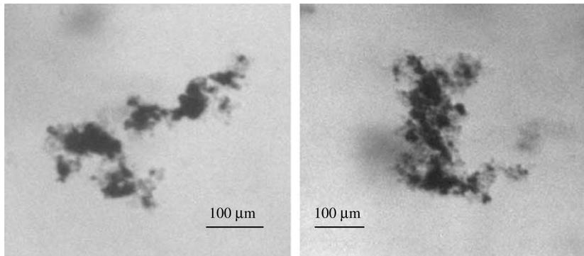
**Figure 2** | *In situ* images of large, porous, loosely bound, highly branched, and irregular aggregates.
