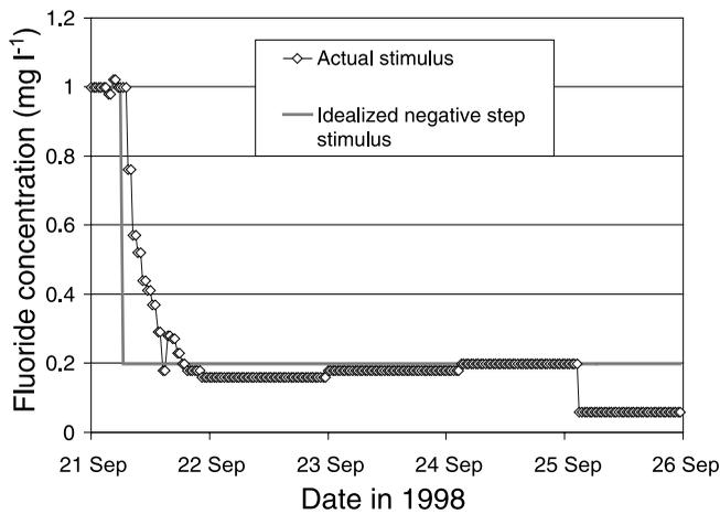
**Figure 4** | Actual pattern of fluoride tracer concentration at leaving the clearwell of E. M. Johnson WTP in Raleigh and the idealized, negative step input used for comparison in the EPANET model.
