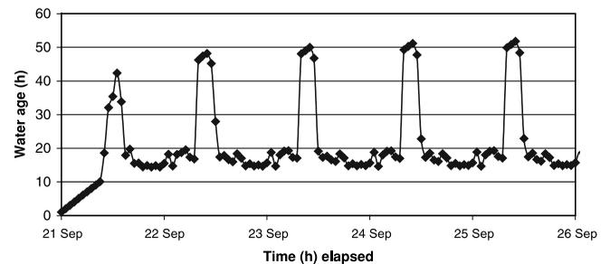
**Figure 7** | EPANET simulation of water age at Southgate Station in Raleigh.
