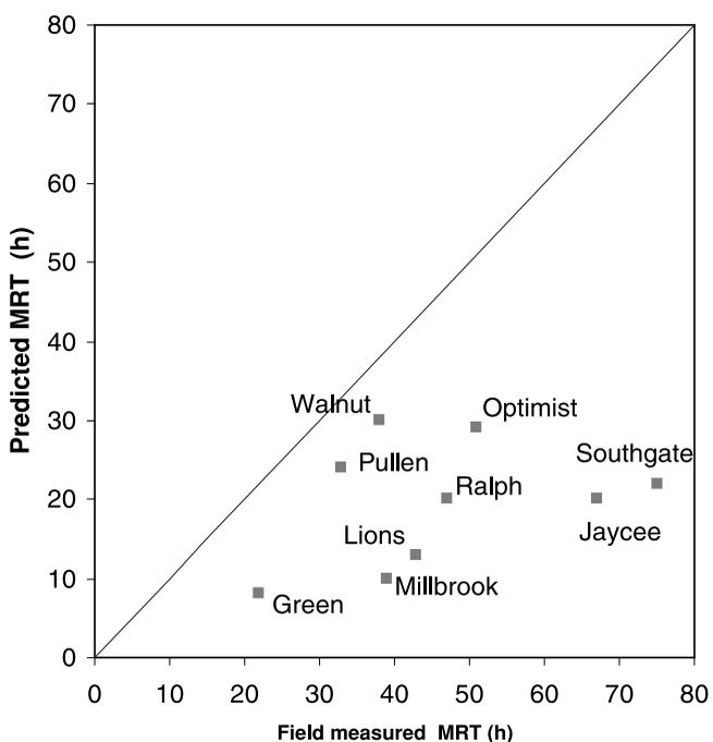
**Figure 10** | Comparison of  $MRT_{model}$  (h) with  $MRT_{field}$  (h) from Raleigh tracer study.
