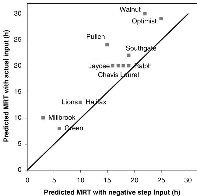
**Figure 6** | Comparison of MRT (h) for actual and negative step input both predicted by EPANET for sampling stations in Raleigh DS.
