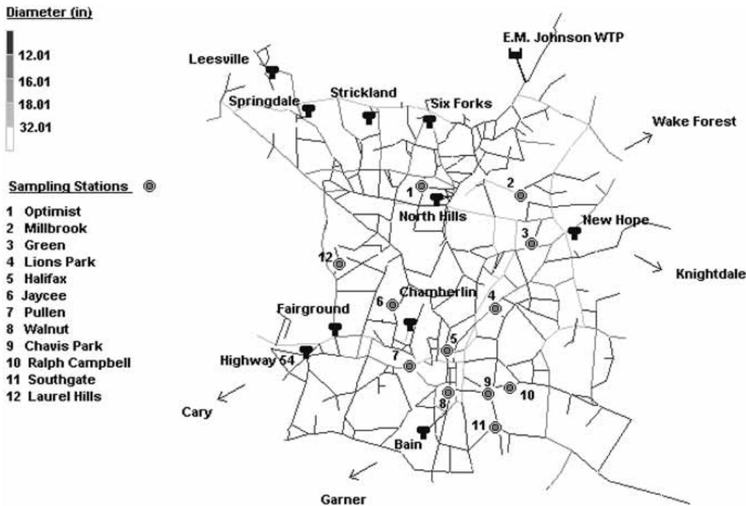
Figure 2 | Skeletonized DS pipe network in Raleigh, North Carolina, showing location of water storage tanks and sampling stations.
