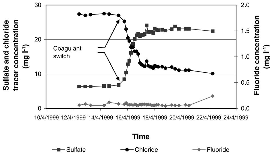
Figure 11 | Tracer concentrations in the finished water at the Brown WTP in Durham.
