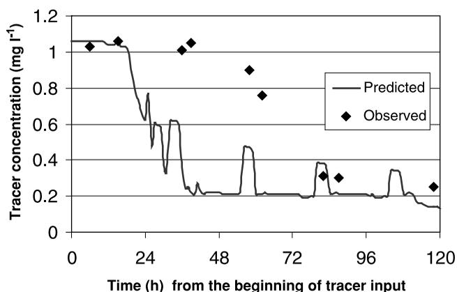
**Figure 9** | Fluoride concentration at Southgate Station in Raleigh as predicted by EPANET and measured during tracer study of September 1998.
