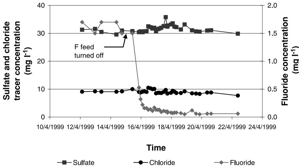
Figure 12 | Tracer concentrations in the finished water of the Williams WTP in Durham.
