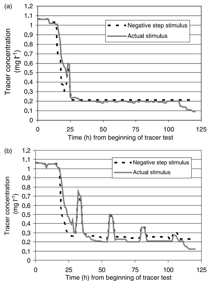
**Figure 5** | EPANET predictions of tracer response at (a) Lions Station and (b) Laurel Station for simulations of both a negative step stimulus and the actual stimulus pattern at E. M. Johnson WTP in Raleigh.
