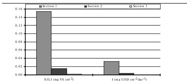
**Figure 6** | Changes in biomass concentration and substrate flux across the biofilter for the conditions of Table 1.
