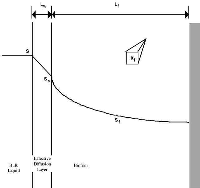
**Figure 2** | Schematic of an idealized one-dimensional biofilm. The z-dimension is perpendicular to the substratum and positive from left to right.
