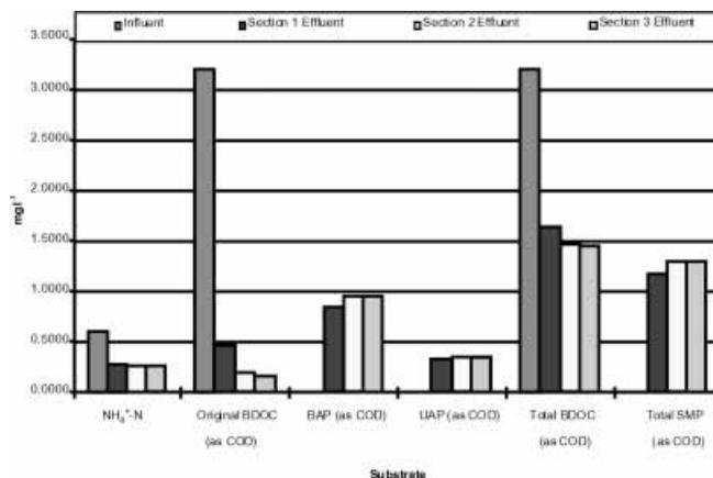
Figure 5 | Changes in the concentrations of the soluble components across the biofilter for the conditions of Table 1.
