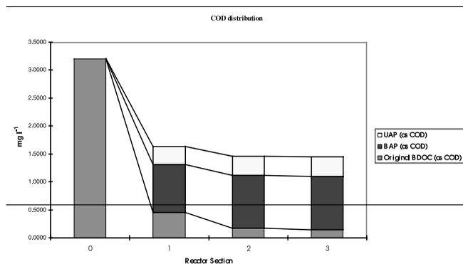
Figure 4 | COD distribution in the reactor for the conditions of Table 1.
