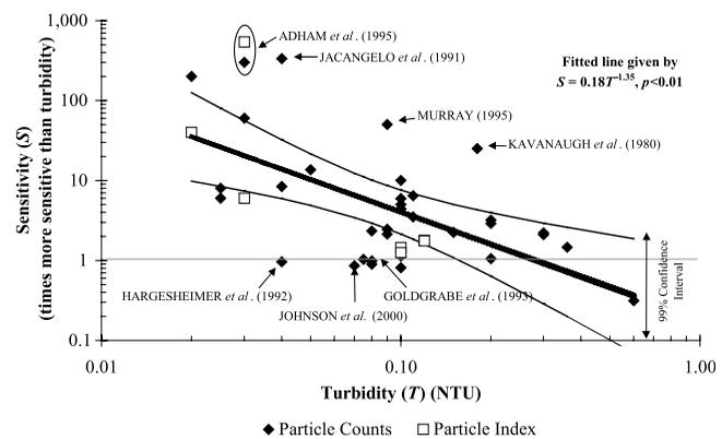
Figure 4 | Particle monitor sensitivity model (literature data).
