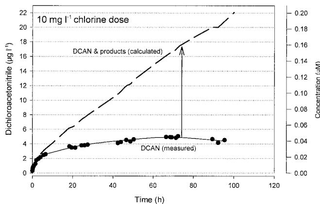
**Figure 13** | Calculated DCAN formation (labelled: DCAN & products) for the chlorination of Thousand Acre Fulvic Acid ( $2.8 \text{ mg l}^{-1}$  TOC) at a chlorine dose of  $10 \text{ mg l}^{-1}$  (pH 7;  $21^\circ\text{C}$ ).
