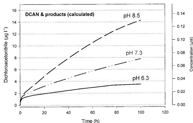
**Figure 14** | Predicted DCAN formation in water from CT utility (11/97) chlorinated at three different pHs.
