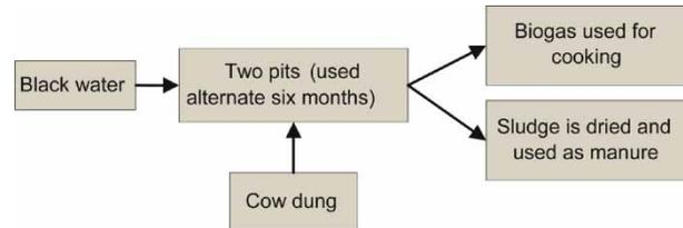
Figure 3 | Outline flow chart of the biogas toilet system.
