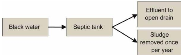
Figure 1 | Outline flow chart of the septic tank system.
