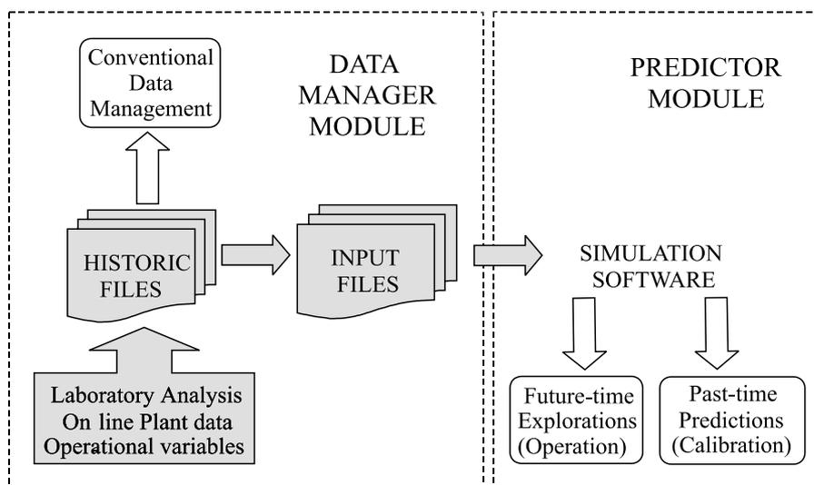
Figure 1 Schematic structure of the modules of the Simulator for Plant Operation
