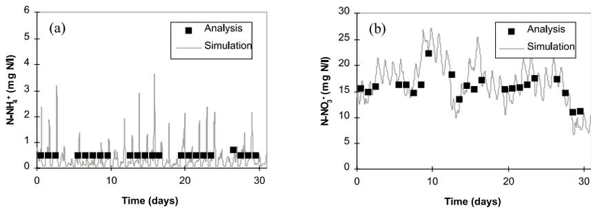
**Figure 5** Real and predicted concentration of ammonia (a) and nitrates (b) in the biological reactors using the calibrated simulator
