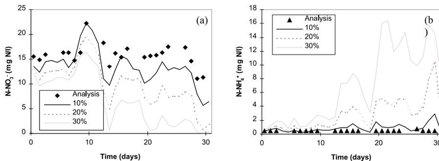
**Figure 6** Effluent quality of WWTP predicted by the simulator of the Badiolegi plant when different percentages (10%, 20% and 30%) of the influent flow are directly introduced to the secondary treatment
