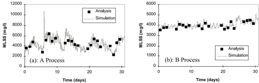
**Figure 4** Real and predicted MLSS concentration in the biological reactors of the A process (a) and the B process (b) using the calibrated simulator
