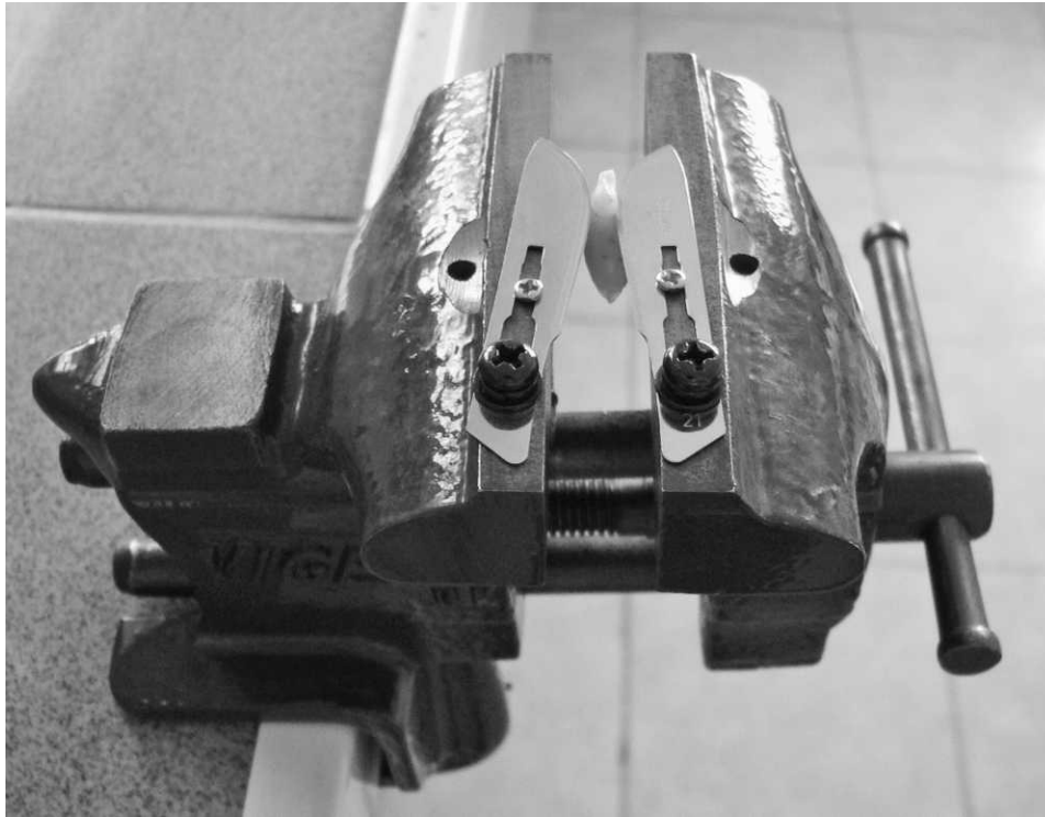
Figure 3. Fracturing device used to fracture the teeth with two surgical blades mounted in a vise, 3 mm from the incisal edge of the incisor.
