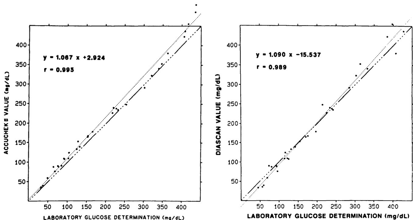
FIG. 3. Relation of Accucheck II (left) and Diascan (2nd evaluation) (right) whole-blood glucose determinations to YSI 23A whole-blood glucose reference determinations (dotted line).
