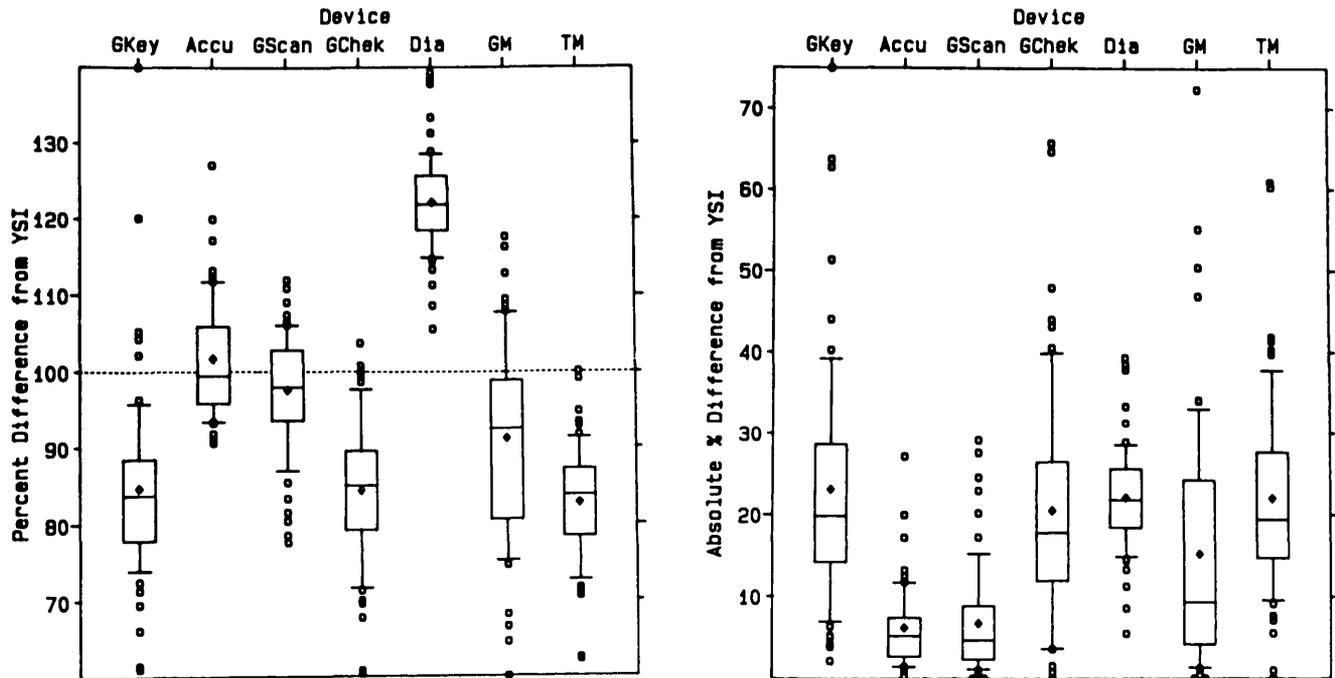
FIG. 2. Distribution of percent differences (left) and absolute percent differences (right) from YSI 23A reference method for Glucokey (GKey), Accucheck bG (Accu), Glucoscan 2000 (GScan), Glucocheck II (GChek), Diascan (Dia), Glucometer II (GM), and Trendsmeter (TM). Boxes span 25–75 quartiles, with median line. Upper and lower bars indicate 90th and 10th percentiles. ♦, Means. Remaining data are plotted.  $n = 56$ .
