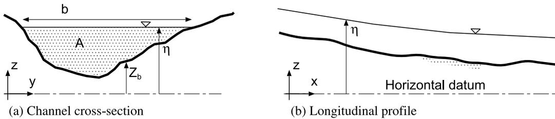
Figure 1 | Definition sketch for narrow channel.
