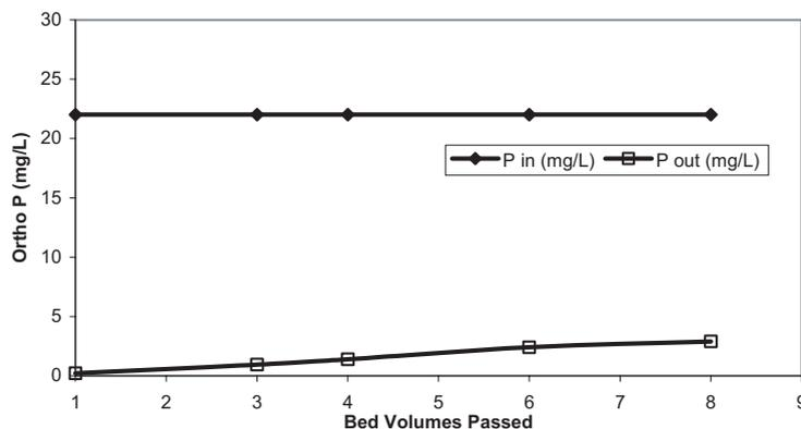
**Figure 7** Breakthrough curve for orthophosphate removal from abattoir wastewater
