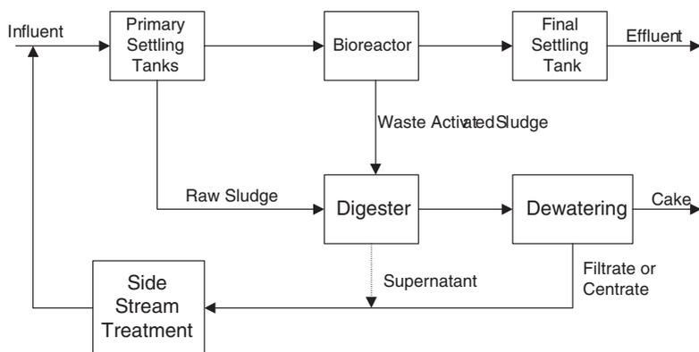
**Figure 1** Typical process flow sheet showing side stream treatment and return to mainstream process
