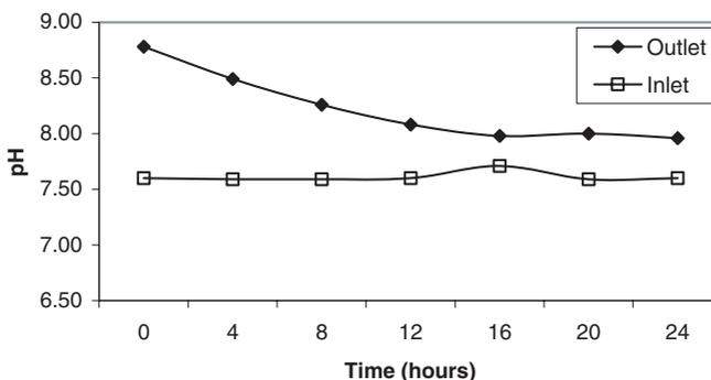
**Figure 6** Typical range of pH values for inlet and outlet solutions during pilot plant operation
