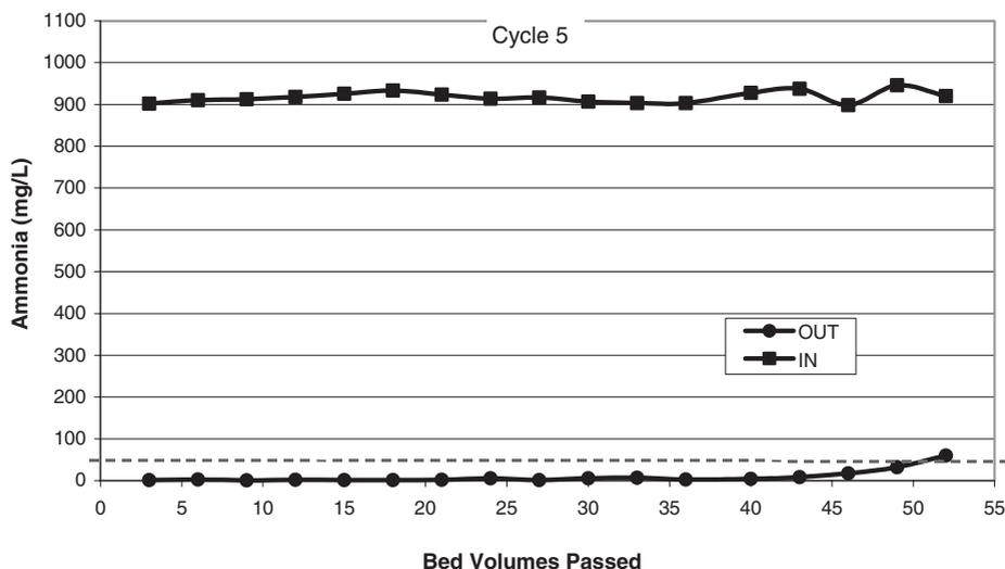
**Figure 3** Breakthrough curve at 1 BV/hour flow rate
