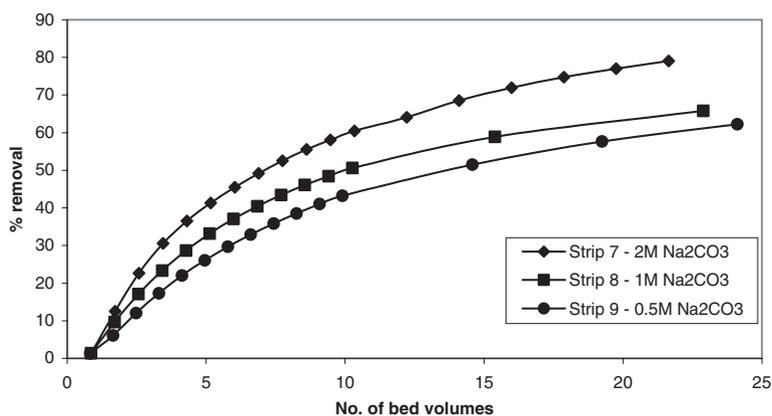
**Figure 4** Summary plot of  $\text{Na}_2\text{CO}_3$  regeneration trials on fully loaded MesoLite
