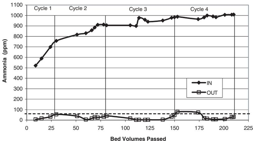
**Figure 2** Typical MesoLite breakthrough curve
