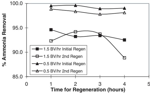
**Figure 5** Efficiency of ammonia removal on successive re-use of  $\text{Na}_2\text{CO}_3$  at different flow rates
