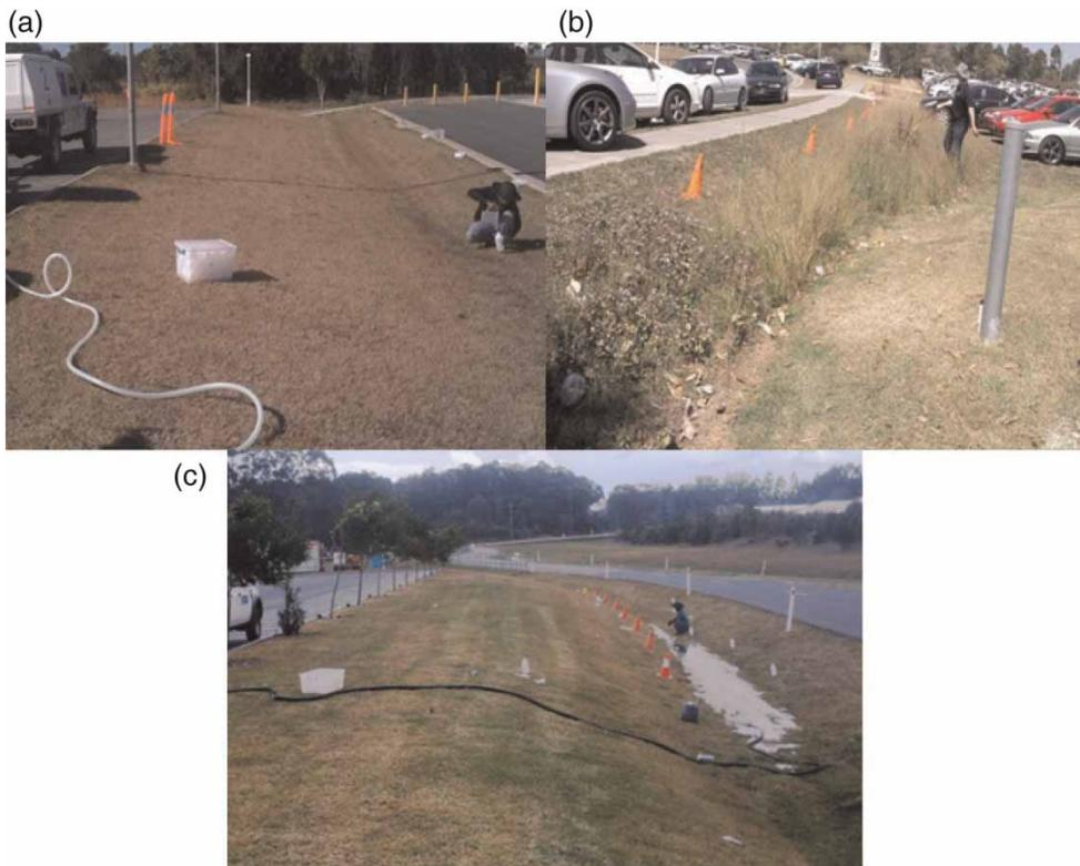
**Figure 1** | Selected swales in the study. (a) Engineering swale – 35 m long, (b) Innovation Centre swale – 30 m long, and (c) Sports Complex swale – 45 m long.
