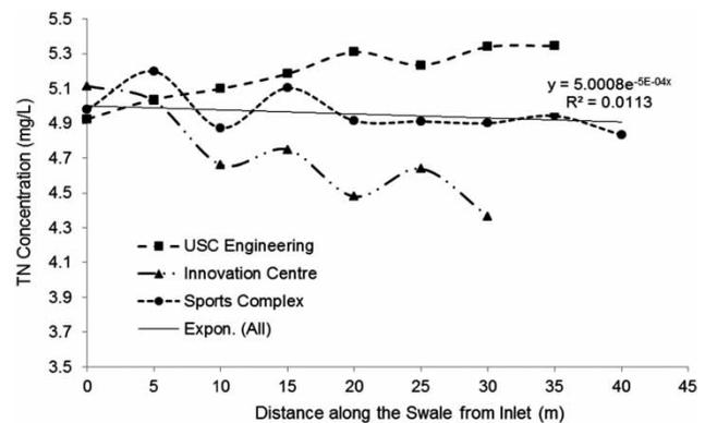
Figure 4 | Reduction in TN along swales for Test C.
