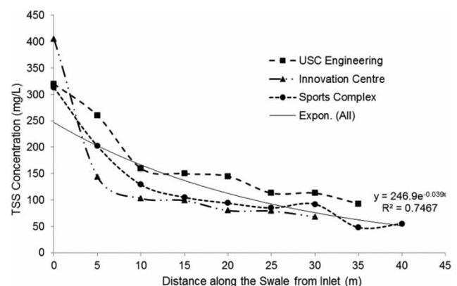
Figure 2 | Reduction in TSS along swales for Test C.
