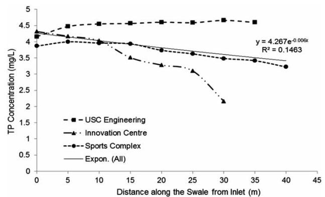
Figure 3 | Reduction in TP along swales for Test C.
