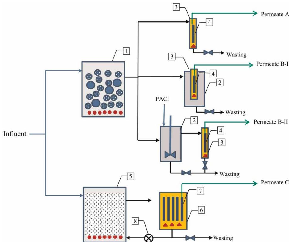
1- MBBR bioreactor; 2- Settling tank; 3-Tertiary filtration membrane tank; 4- Membrane module;
