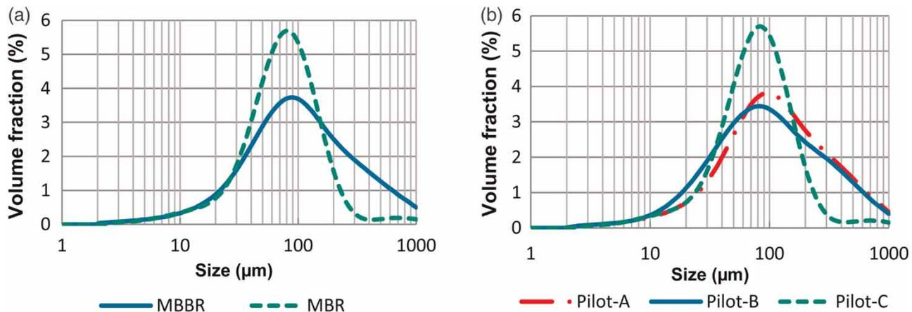
Figure 4 | Particle size distribution of the mixed liquor in (a) bioreactors and (b) membrane tanks.
