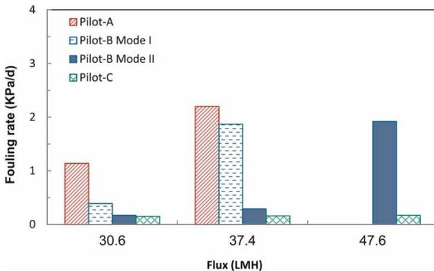
Figure 3 | Comparison of fouling rates between three pilot units.
