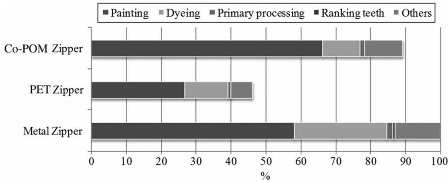
Figure 4 | IWF percentage of the different production processes.
