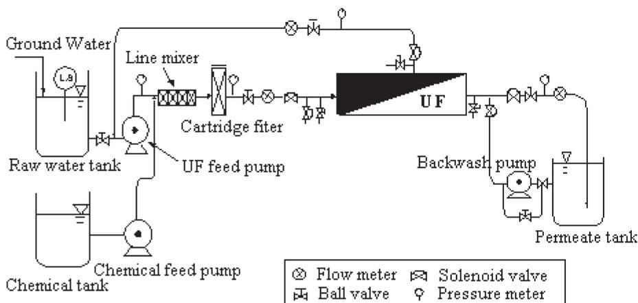
**Figure 2** Schematic diagram of UF membrane pilot plant
