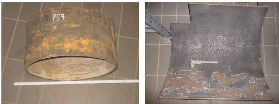
Figure 3 | Samples of a DN 500 (left) and a DN 700 (right) trunk main.
