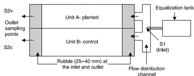
Figure 1 | Schematic diagram of the HSSF-CW pilot plant.
