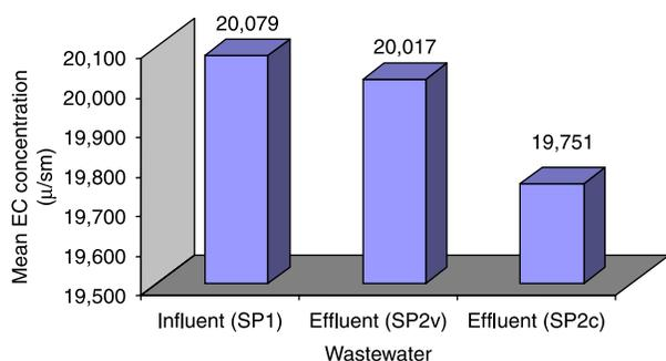
**Figure 7** | Mean values of EC concentrations in the Mesocosms.
