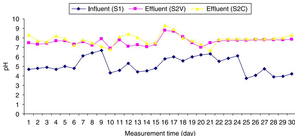
**Figure 5** | Variation of pH at the inlet and outlet of vegetated and control cells.
