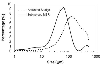
**Figure 2** Size distribution of the sludge from a conventional plant and submerged MBR
