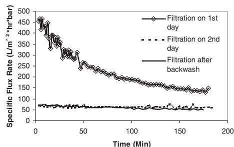
**Figure 4** The deterioration of filtration performance
