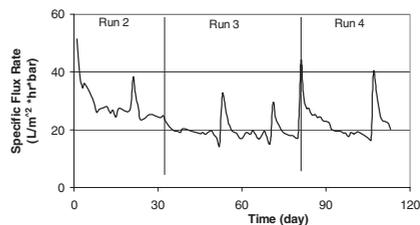
**Figure 3** Filtration performance of submerged MBR
