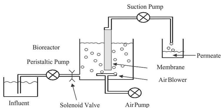
**Figure 1** Schematic diagram of the submerged tubular ceramic membrane bioreactor
