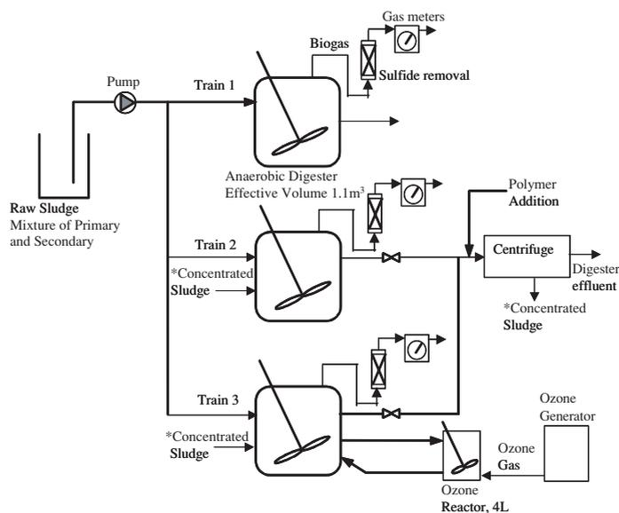
**Figure 1** Process configuration for different experimental trains
