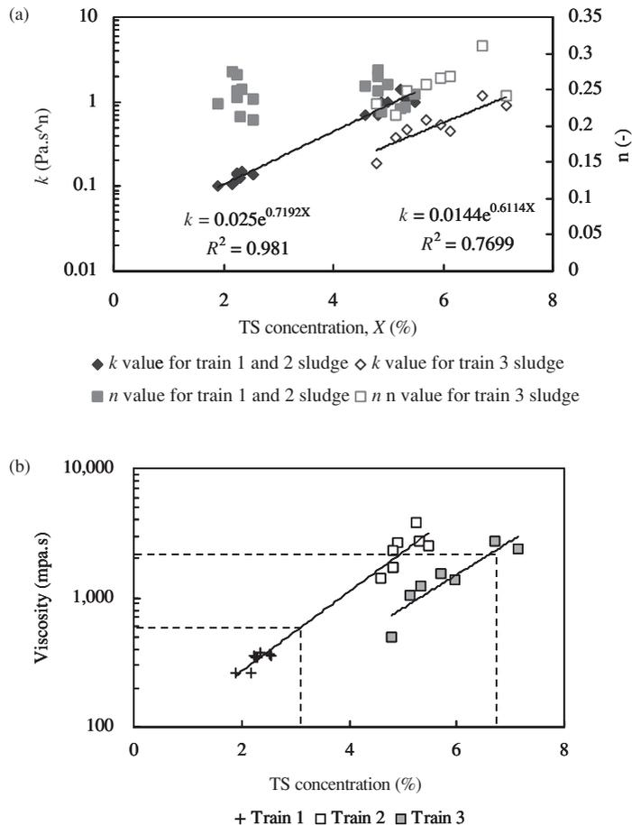
**Figure 3** (a) Non-Newtonian viscosity parameters; (b) change in viscosity with TVS concentration
