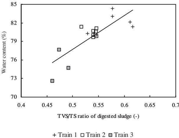
**Figure 5** Relationship between water content in dewatered sludge and TVS/TS
