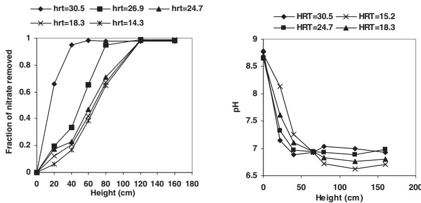
**Figure 2** Effect of hydraulic retention times (HRTs) on  $\text{NO}_3^-$  removal and pH profiles in the column reactor inoculated with *T. denitrificans* MP
