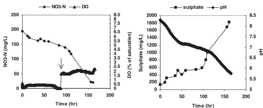
**Figure 5.** Concentration profiles of  $\text{NO}_3^-$ , saturation of DO,  $\text{SO}_4^{2-}$  and pH in the fermenter system when the initial DO was 1.3% of saturation and adjusted to between 1.7 and 2.1 indicated by an arrow
