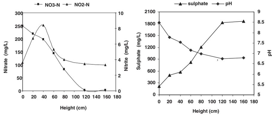
**Figure 1** Sulphate ( $\text{SO}_4^{2-}$ ), nitrate nitrogen ( $\text{NO}_3^-$ -N), nitrite nitrogen ( $\text{NO}_2^-$ -N) and pH profiles within the column reactor packed with sulphur particles and limestone granules and fed with synthetic wastewater at an upflow rate of 0.5 L/hr
