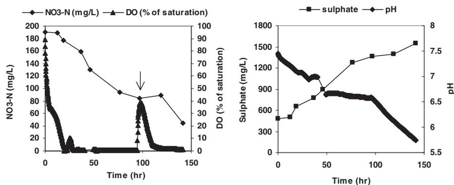
**Figure 4.** Concentration profiles of  $\text{NO}_3^-$  and sulphate, saturation of DO and pH in the fermenter system. Note the surge of DO at 97.8 hrs (indicated by an arrow) by manipulation and the slow down of denitrification
