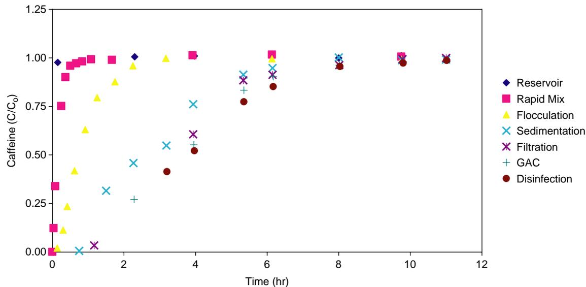
Figure 3 | Breakthrough curves for caffeine in blank system.
