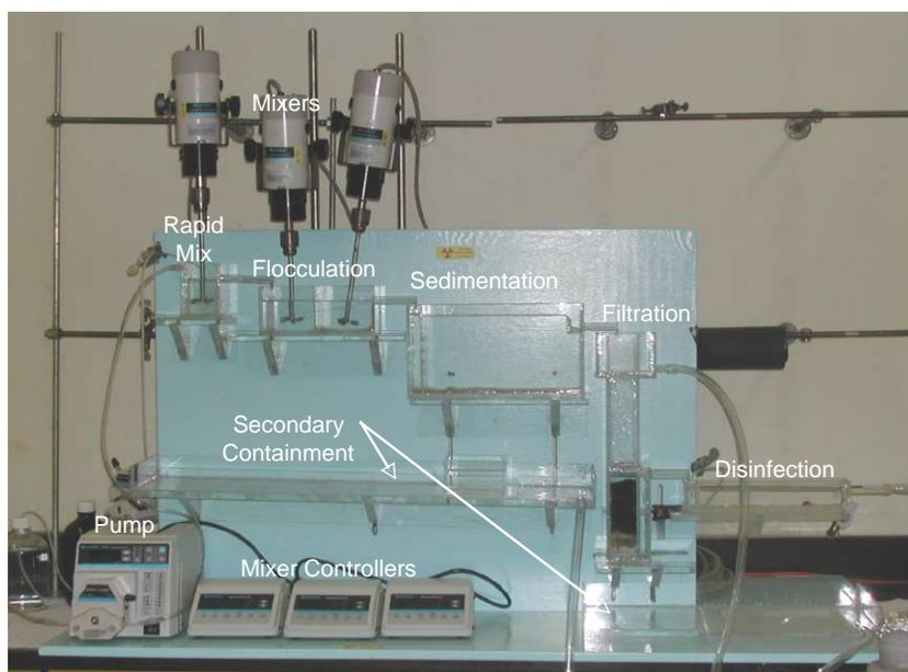
Figure 1 | Photograph of bench-scale drinking water treatment plant.
