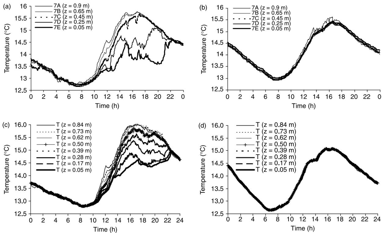
**Figure 3** | Temperatures measured (a and b) and simulated (c and d) at site 7 with stratification (03/18/2005, a and c) and without stratification (03/31/2005, b and d).
