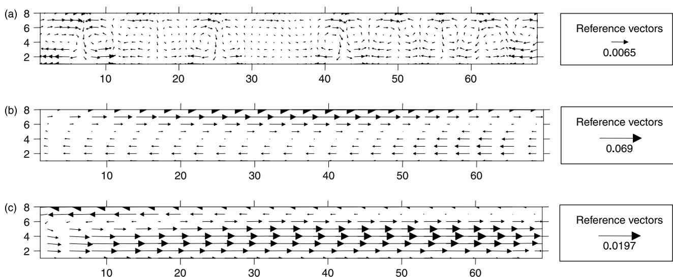
**Figure 4** | Velocity field cross-sections at  $x = 190 \text{ m}$ . Vertical mixing in convection cells on 03/17/2005 at 00:10 am, with a wind speed equal to  $0.8 \text{ m s}^{-1}$  (a). Strong wind conditions, with a wind speed of  $8 \text{ m s}^{-1}$  on 03/31/2005 at 10:00 am (b). Low influence of wind ( $2.5 \text{ m s}^{-1}$ ) on the 03/18/2005 at 3:00 pm (c). Space coordinates unit: m. Reference vectors unit:  $\text{m s}^{-1}$ .
