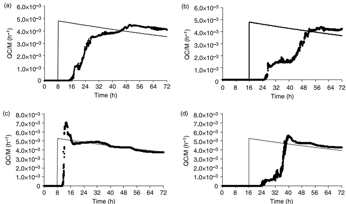
**Figure 5** | Simulated RTD for runs 1 (a) to 4 (d). The CSTR curve (thin line) is plotted on each graph for comparison. Q = flow rate; C = tracer concentration; M = injected mass.
