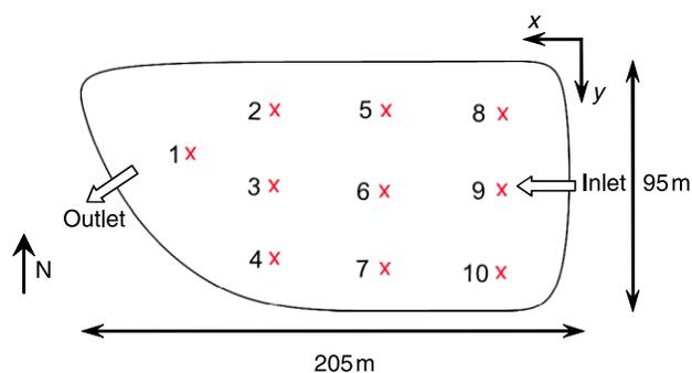
Figure 1 | Layout of the pond and location of the 10 temperature measurement sites.
