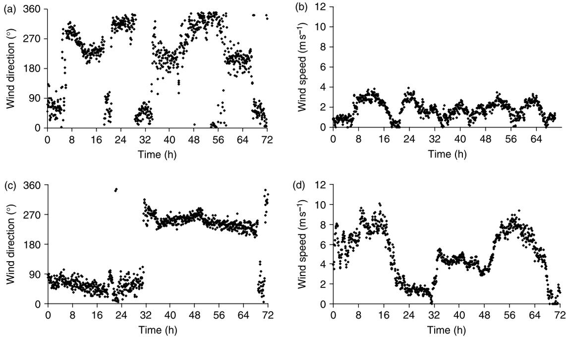
**Figure 2** | Wind speed and direction recorded at the Mèze WWTP for 3 days from 03/18/2005 (a and b) and 03/31/2005 (c and d) at 00:00 am. Wind direction: N = 0 = 360, W = 90, S = 180, E = 270.
