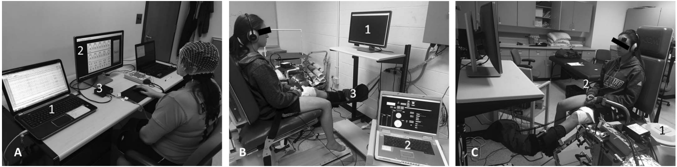
Figure 2. A, Setup for measure of emotional response. A1, Electroencephalograph; A2, Self-Assessment Manikin; A3, Electrocardiogram. B and C, Setup for stiffness testing in response to emotionally evocative pictures. B1, Picture presentation screen; B2, SPAD control computer; B3, Vacuum splint. C1, SPAD machine; C2, Safety switch. SPAD, a custom-built stiffness- and proprioception-assessment device.
