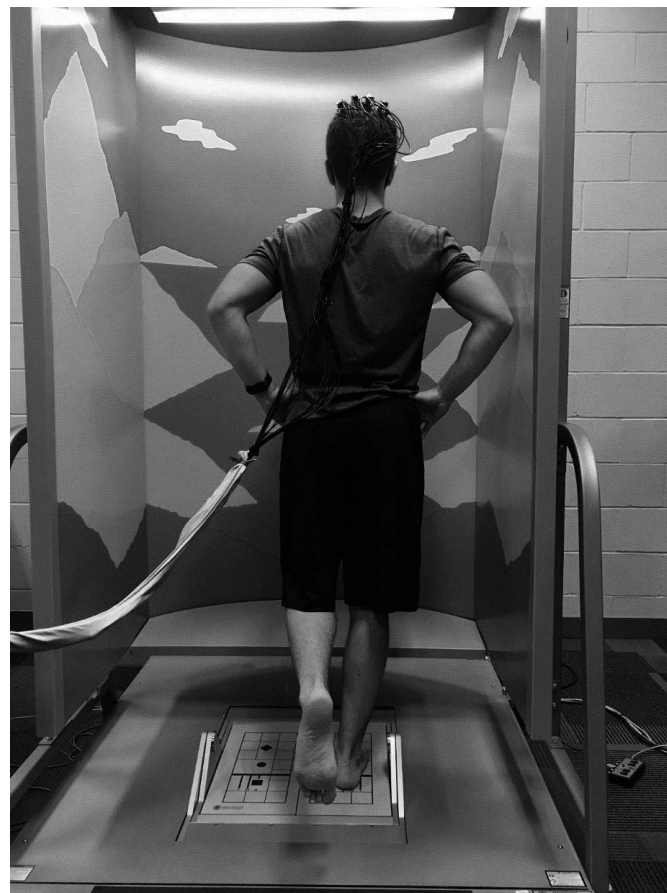
Figure 1. Testing setup on the force platform (Balance Master System 8.4; NeuroCom, Clackamas, OR) with the functional near-infrared spectroscopy system affixed to the head.
