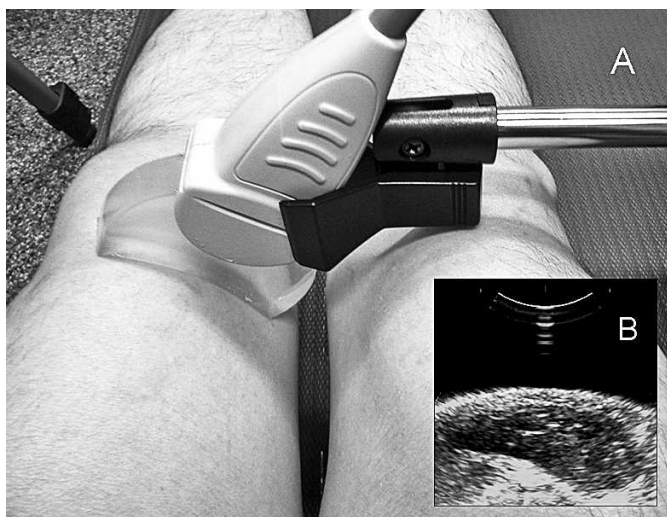
Figure 2. A, Hands-free ultrasound imaging. B, Corresponding ultrasound image. The laser provided a reference for positioning the participant and locating the vastus medialis obliquus.
