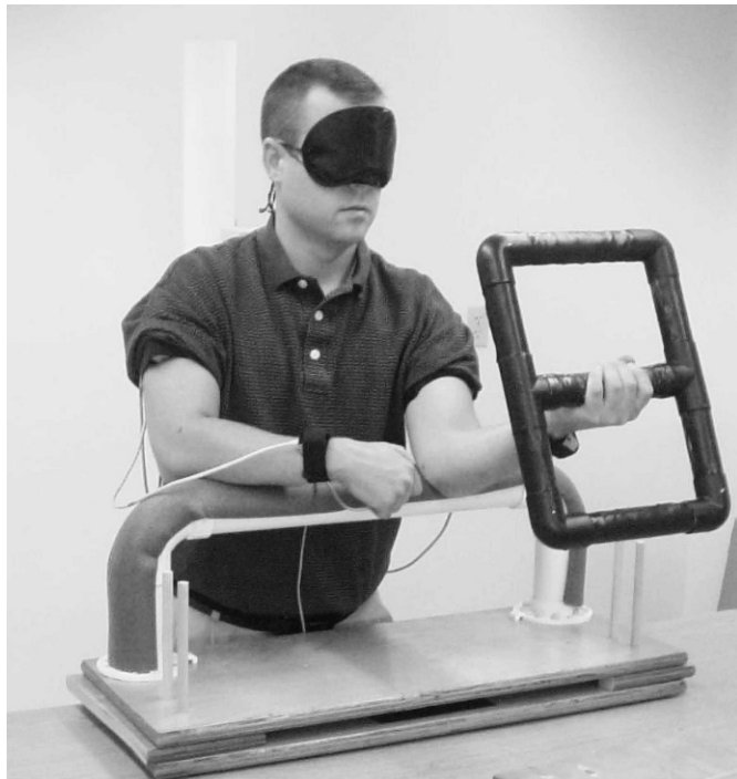
Figure 2. A blindfolded participant holds a dumbbell and attempts to reproduce the elbow flexion angle during joint position sense testing.
