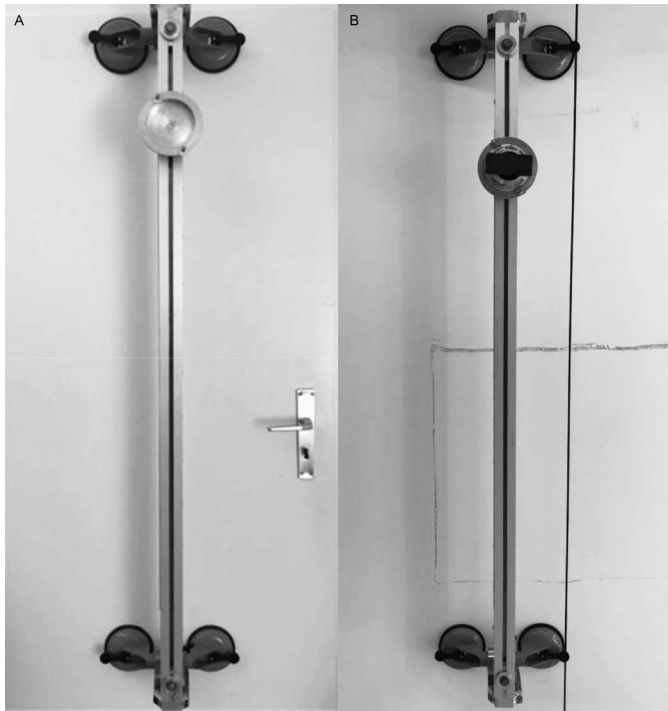
Figure 1. The Self-Assessment Corner, A, without and, B, with the handheld dynamometer placed in the receptacle.
