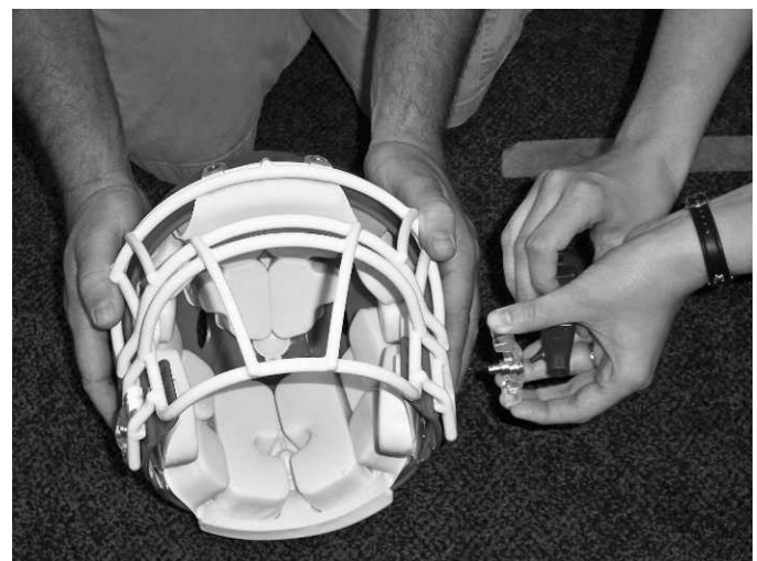
Figure 3. Football helmet stabilization and Quick Release Face Guard Attachment System (Riddell Sports, Inc, Elyria, OH) clip removal. Manual stabilization of the helmet was performed to mimic helmet-stabilization techniques used during an emergency situation. For clip removal, one hand was used to manipulate the tool, and the other hand provided stabilization and pulled the clip from the helmet after release of the locking-pin mechanism.
