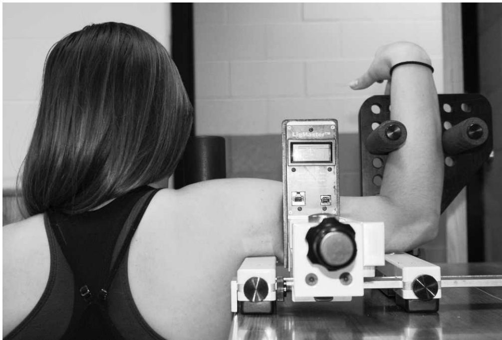
Figure. Measurement of anterior glenohumeral laxity using the instrumented arthrometer.
