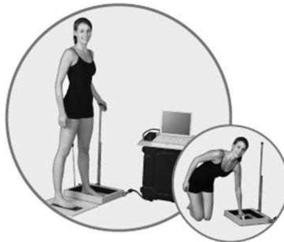
**Figure 1. Perometer.** A perometer uses arrays of light switches made up of light-emitting diodes to illuminate, scan, and calculate the volume of an extremity in milliliters (mL). Lower leg volume was calculated from the medial malleolus to the tibial tuberosity and was measured with the participant in a standing position. Reprinted with permission from [www.pero-system.de](http://www.pero-system.de).
