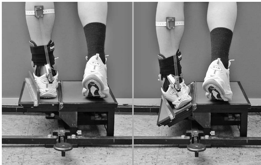
Figure 2. Simulation of an ankle sprain (foot inversion) on the tilting platform (30° tilting dislocation) measured with the in-shoe goniometer system. The left leg and foot are fully loaded. Here, the braced condition is illustrated.
