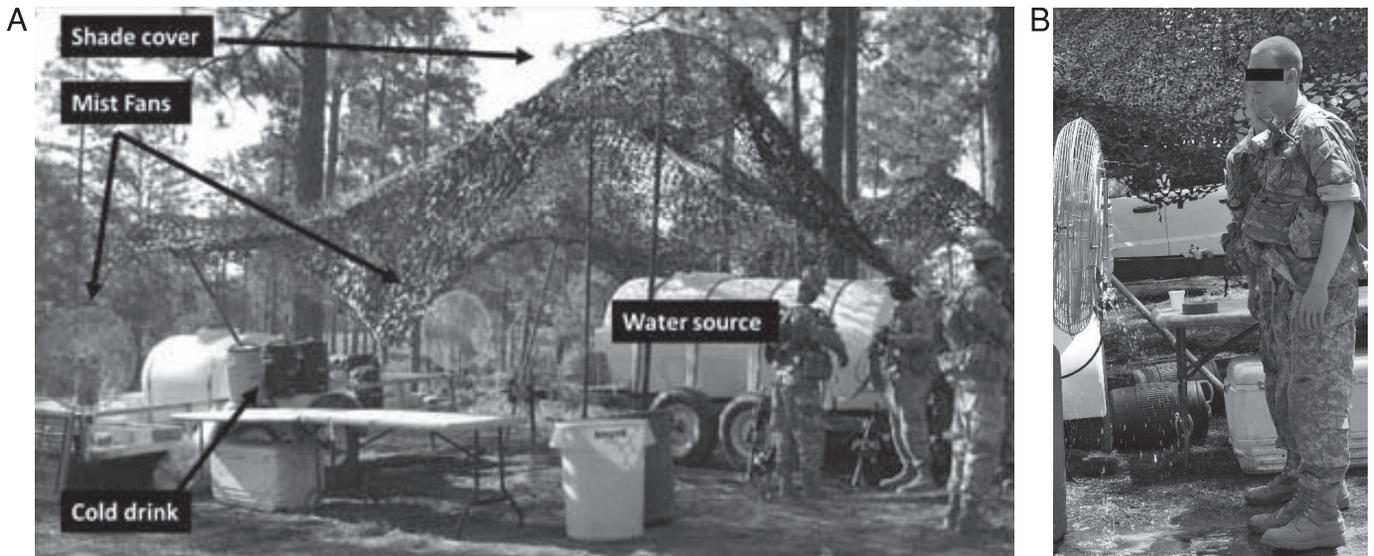
Figure 1. A, Cooling zone setup. B, Mist fan.
