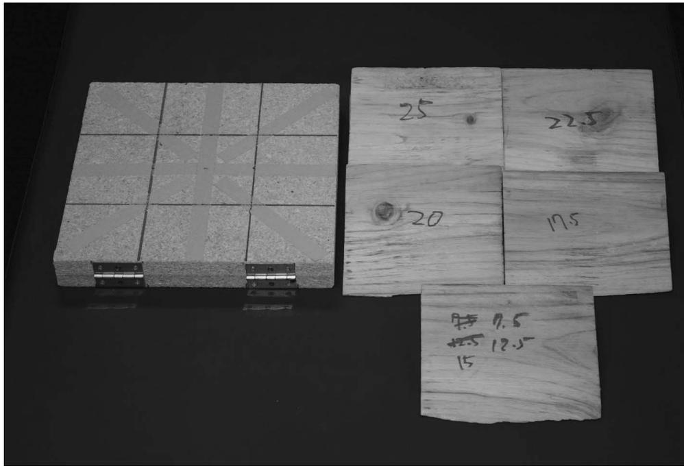
Figure 2. Slope surface board and angle wedges.
