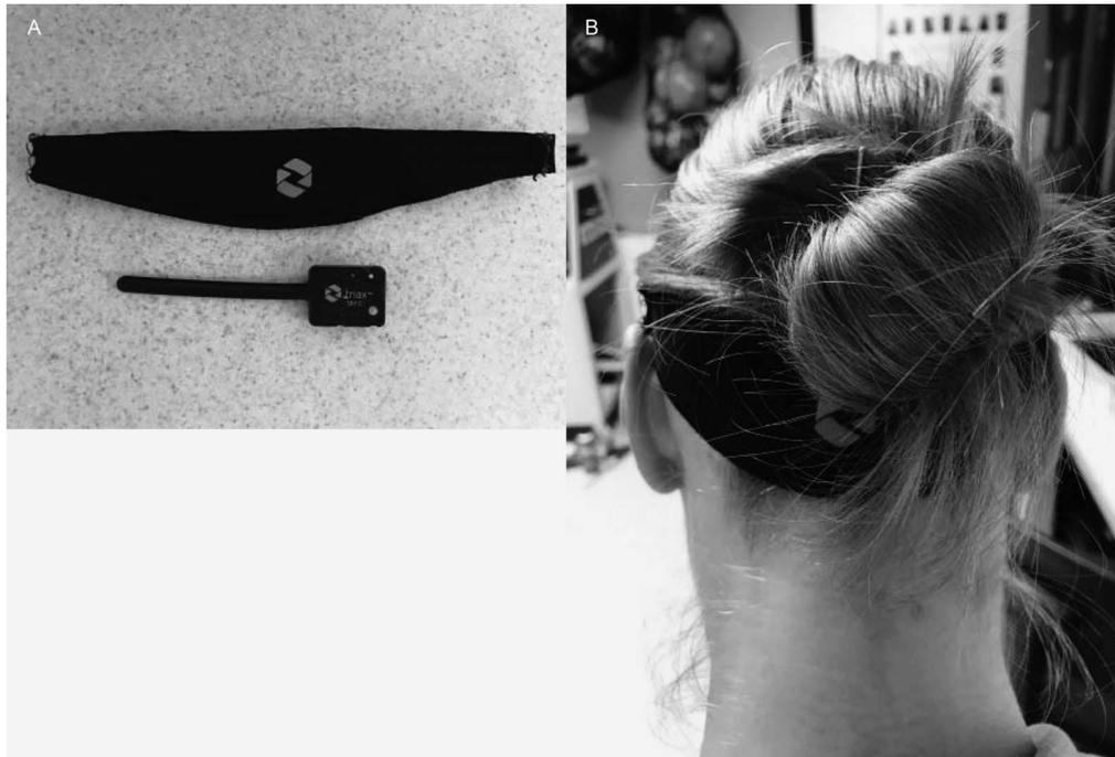
**Figure 1.** Smart Impact Monitor (firmware version 3.7; SIM-G, version 3.3; AP, version 0.9.150413; software, Triax Technologies, Norwalk, CT) with A, custom headband, and B, placement of the headband on the head.
