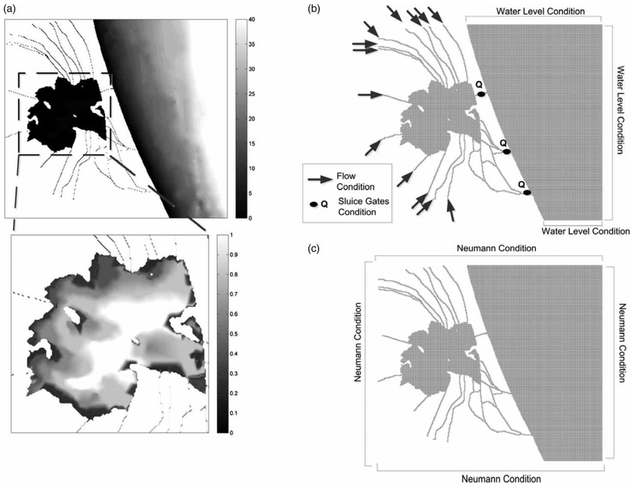
**Figure 3** | (a) Hydrodynamic model grid of the whole aquatic system (irrigation channels, lagoon, 'golas' and Mediterranean Sea). (b) Boundary conditions of long wave model. (c) Boundary conditions of wind model.
