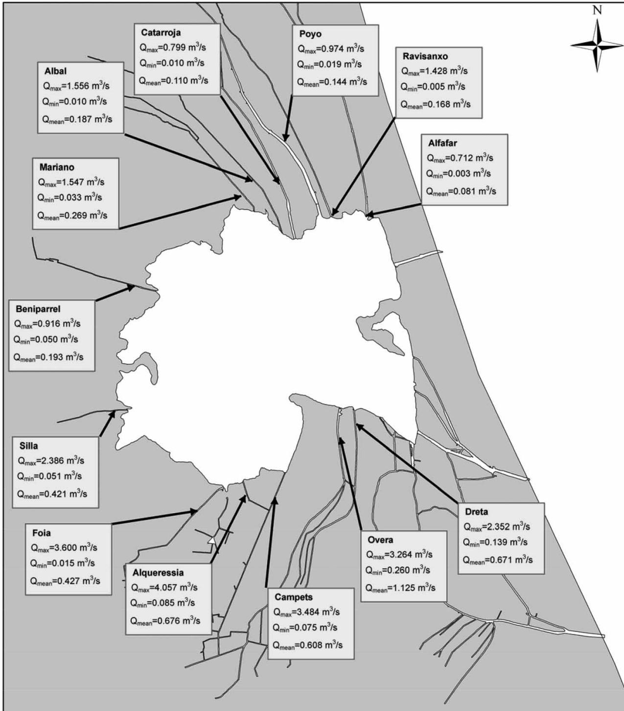
Figure 6 | Maximum, minimum and mean value of irrigation channel discharges into the lagoon from October 2005 to September 2006.
