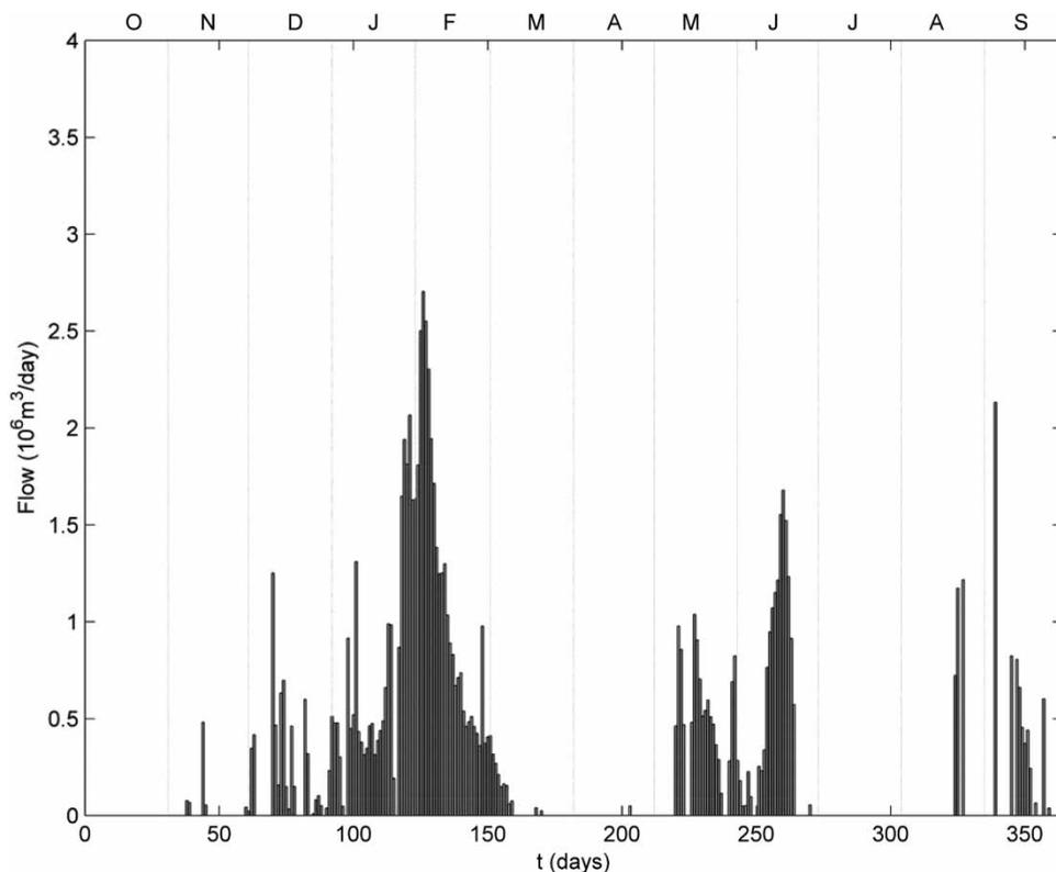
**Figure 11** | Daily lagoon outflows through the sluice gates.
