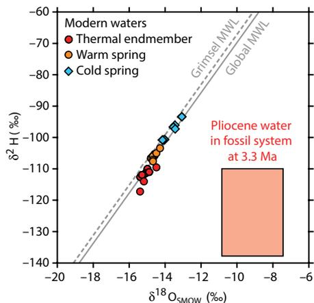
**Figure 2. Stable O-H isotope signatures of cold and warm springs and reconstructed end-member thermal waters, all showing close association with meteoric water lines (MWL). Rectangle denotes isotope signatures of fossil system at 3.3 Ma (Hofmann et al., 2004), consistent with meteoric water origin. SMOW—standard mean ocean water.**
