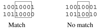
Figure 2: Using the r -contiguous bits matching rule with r = 4 , the two strings on the left constitute a match. The two on the right, with a maximum of 3 matching contiguous bits, do not match.
