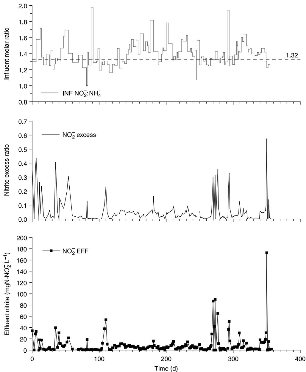
**Figure 2** | The influent nitrite to ammonium molar ratio contrasted with the nitrogen nitrate effluent concentration and the corresponding nitrite excess.
