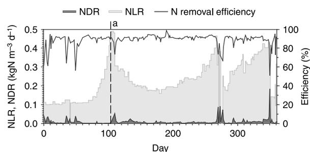
**Figure 1** | Process performance in terms of Nitrogen Loading Rate (NLR) and Nitrogen Discharge Rate (NDR), with the corresponding nitrogen removal efficiency. (a) New leachate.
