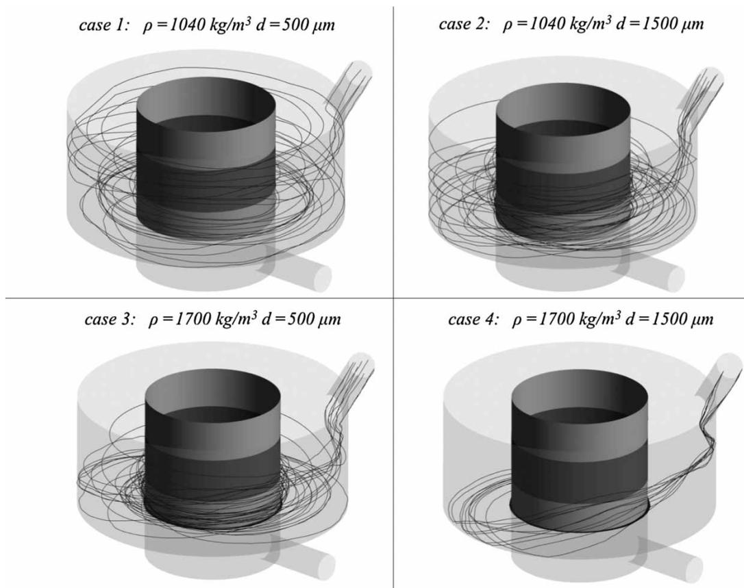
**Figure 3** | Trajectories of 10 particles using the global scale model for a flow rate equal to 25 L/s.
