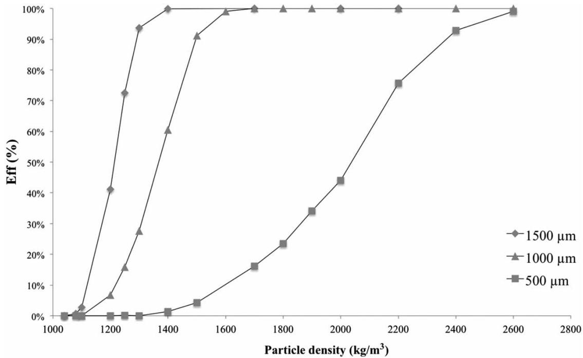
**Figure 2** | Particles trapping efficiency (Eff) with the conceptual porous screen ( $Q = 25$  L/s) for different particle densities and diameters.
