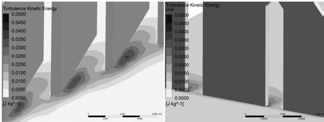
**Figure 4** | Turbulence kinetic energy field for two different screens for an equivalent flow rate of 25 L/s: expanded-metal screen (left) and perforated plate with hexagonal holes (right).
