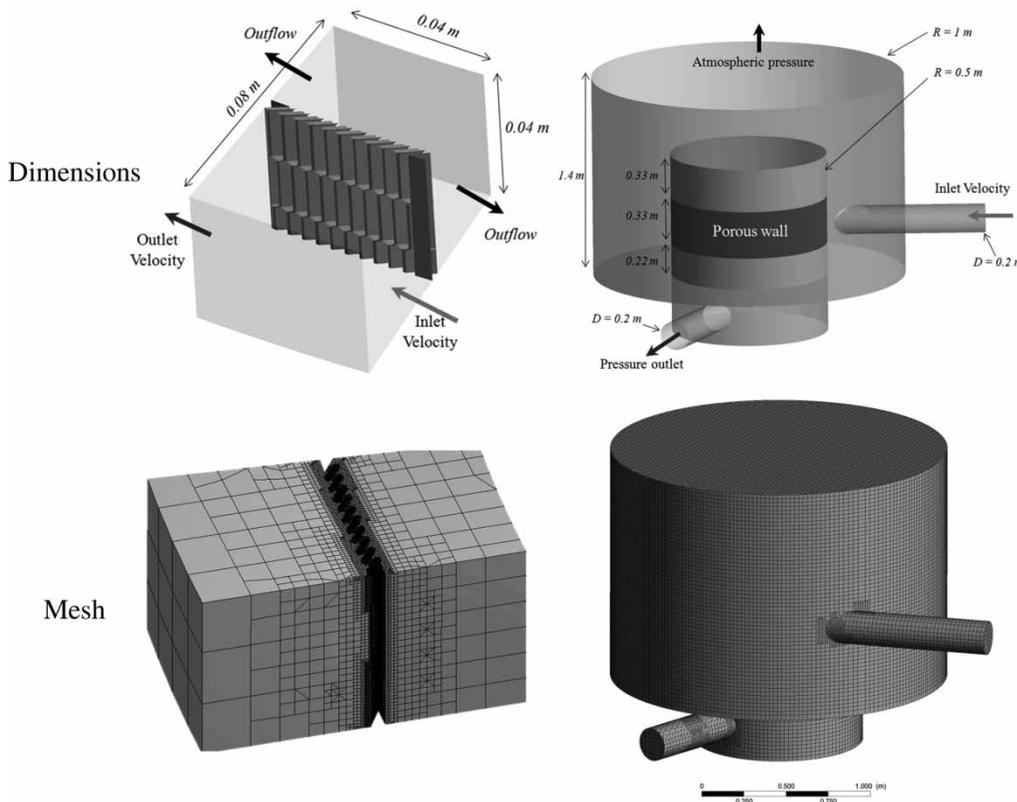
Figure 1 | Dimensions, hydraulic conditions and mesh discretization for the local scale model and for the global scale model.
