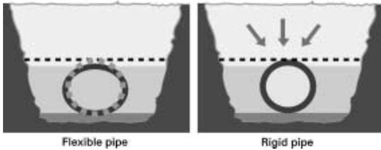
Figure 4 Consolidation of the sidefill gives increased deflection in flexible pipes and an increased load on rigid pipes
