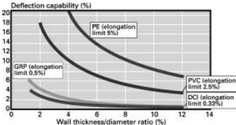
Figure 6 Deflection capability as a function of wall thickness/diameter ratio
