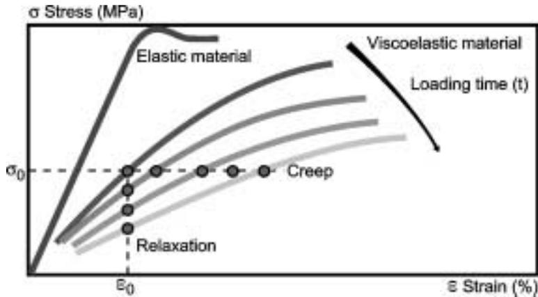
**Figure 1** Stress/strain relationship for elastic and viscoelastic materials
