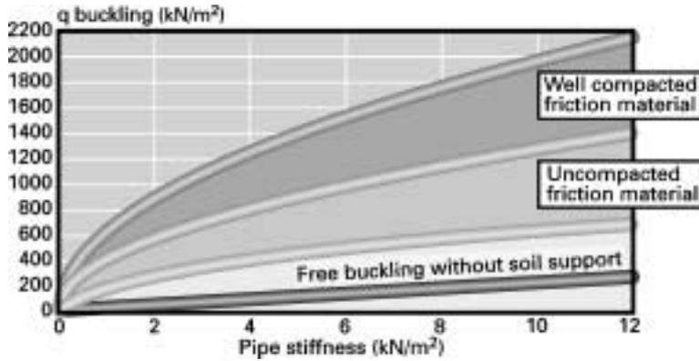
Figure 3 Buckling resistance as a function of pipe stiffness
