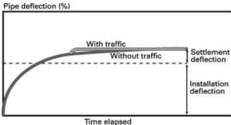
Figure 7 Typical deflection of a buried flexible pipe as a function of time
