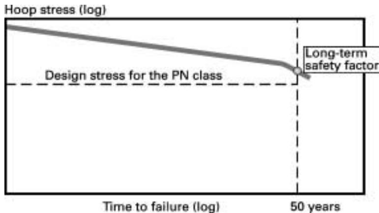
**Figure 2** Schematic creep rupture curve for a thermoplastics pipe
