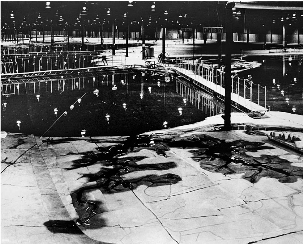
Figure 5. The sprawling Chesapeake Bay Hydraulic Model, housed in a warehouse that covered fourteen acres, became obsolete as soon as construction was finished. Photo courtesy of the US Army Corps of Engineers
