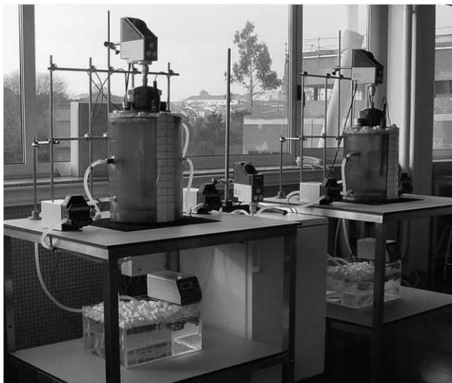
**Figure 1** Anaerobic digestion pilot plant
