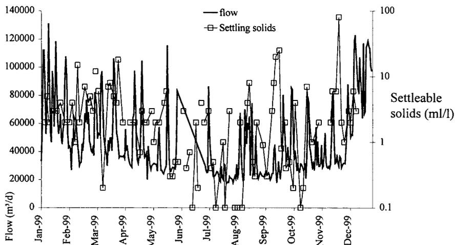
**Figure 3** Settleable solids measurements versus flow (90 measuring points)
