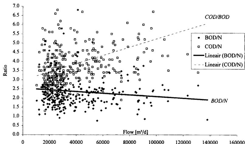
**Figure 2** COD/BOD and BOD/TN versus flow (376 measuring points)
