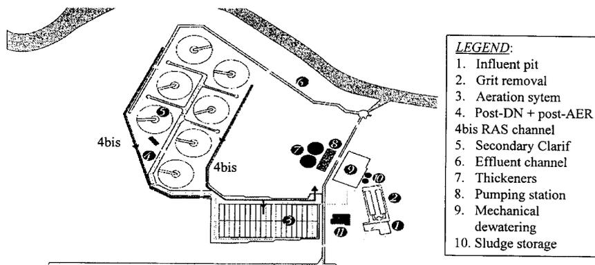
**Figure 1** Plant layout of the STP of the city of Ghent
