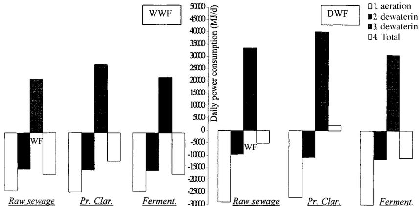
**Figure 4** Simulated energy balance, expressed in  $\text{MJ}\cdot\text{d}^{-1}$ : (a) WWF, (b) DWF
